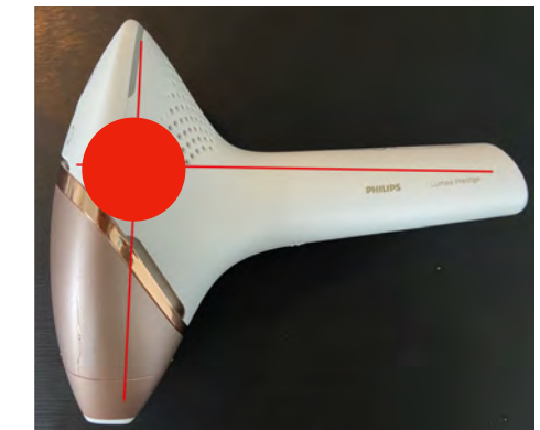
Figure 17 Estimated centre of mass of Philips IPL device
