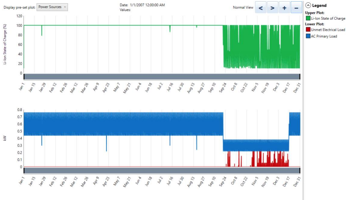
Figure 31. BESS SoC vs. total electrical load and unmet electrical load.
