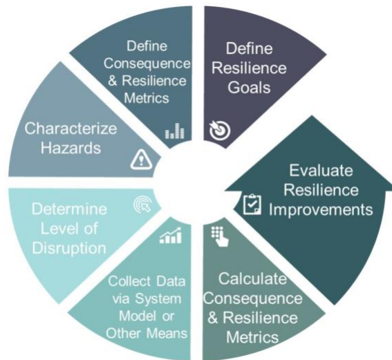
Figure 5. The Resilience Analysis Process' steps move on counterclockwise starting from "define resilience goals" [28].
