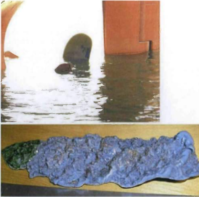
Figure 15 Composite image of a replica of erosive damage in the Trailing Edge region of the propeller blade, as indicated on the emerged propeller blade with marker paint (Courtesy Lloyd's Register)
