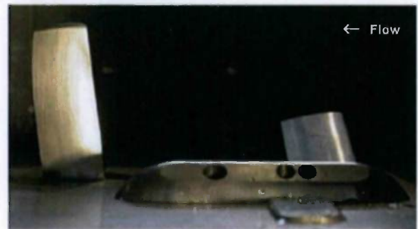
Figure 8 Side view of experimental setup. The test fin is on the left, the vortex generation fin is on the right. Flow is right to left (Moeny et al. [17]).
