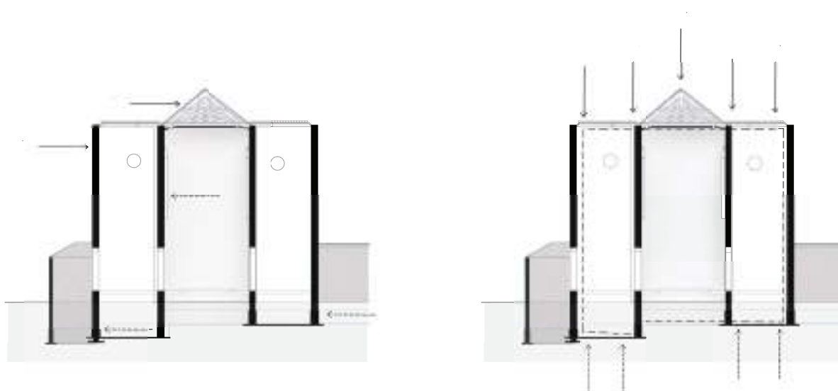
Vertical and horizontal forces transmission scheme section c
