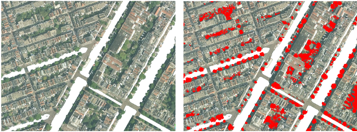
Figure 4.11: Points in an example scene classified as vegetation when NDVI = 0.1 (classified points in red).
