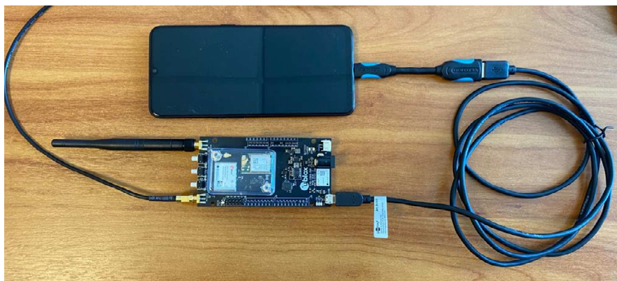
Figure 3.7: Connection between application board and smartphone
