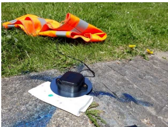
Figure 3.5: The GNSS antenna set-up
