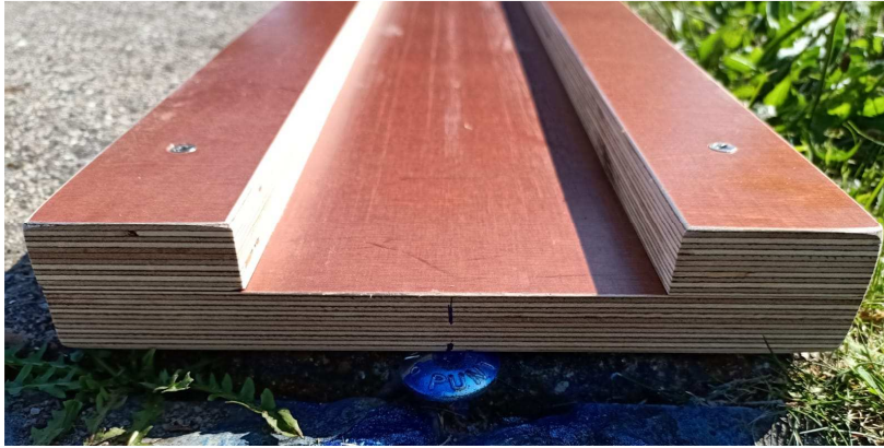
Figure 3.10a-c: a-b) Positioning of the track right above benchmark 2. c) Positioning of the start of the track right above benchmark 1.
