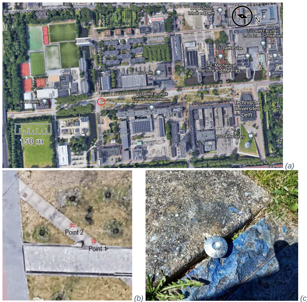
Figure 3.2a-c: a) The location of the reference points on the TU Delft campus, located to the south-east of the city centre, indicated by the red circle; b) The exact location; c) One of the benchmarks
