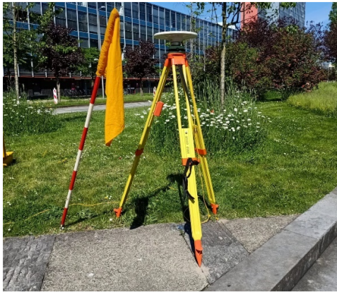
Figure 3.3: Trimble antenna and tripod
