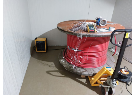
(b) 415m of Telcon XLPE cable, 1x25mm 2 with Aluminum conductor and a 16mm 2 cross section of the screen.
