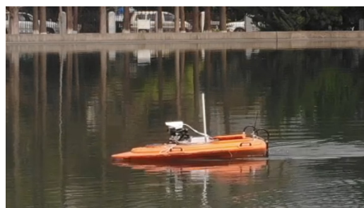
Figure 8. The twin-propulsion ASV used for modeling in simulation experiments.
