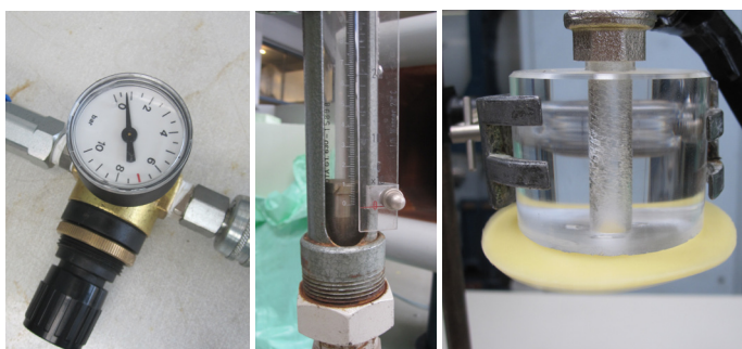
Figure 9: Left: Air regulator. Middle: Flow sensor. Right: Bernoulli gripper in the clamp gripping an object.
