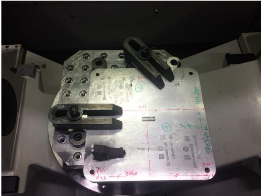
Figure 8.3: Clamping of the base plate to fix the part in the CNC machine
