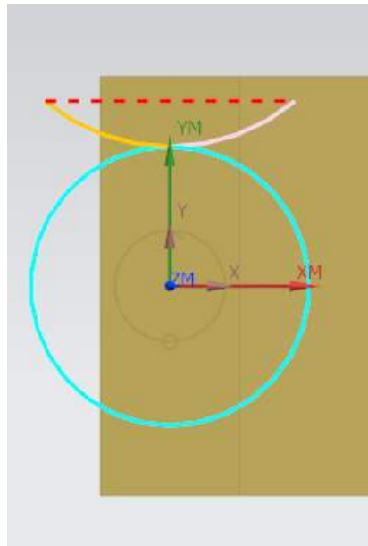
Figure 8.6: Reference point and machining operation of pin 1 on the side
