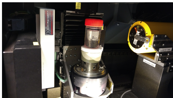
Figure 6.4: XCT setup for the evaluation of sealing effect of WSRP in mortar.
