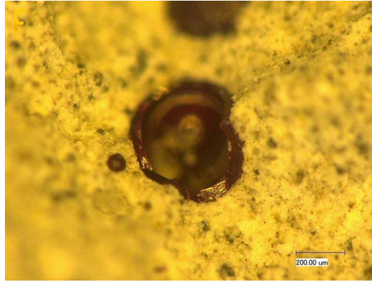
Figure 3.15: OM image of fracture surface with a ruptured microcapsule triggered by crack propagation.
