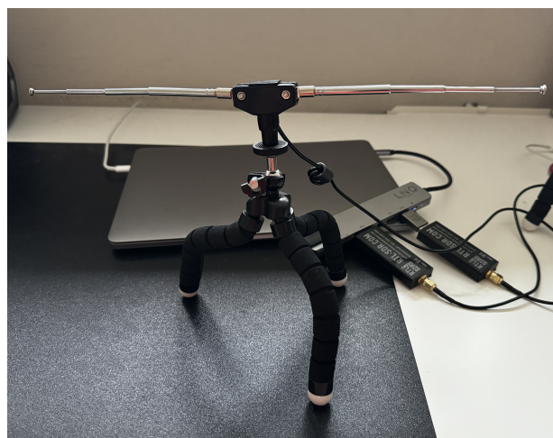
Figure 14: Figure showing the prototyping hardware antenna setup.
