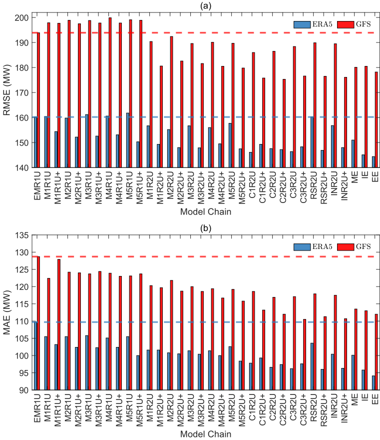
Figure 4.8: Neural network wind power model chains compared with the empirical model: (a) RMSE, and (b) MAE. For ease of comparison, the horizontal dashed lines show the error for the empirical model (EMR1U) using ERA5 (blue) and GFS (red) as input.
