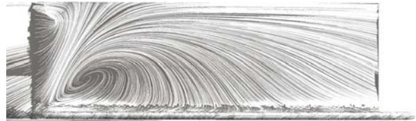
Figure 13. Surface flow pattern obtained with Spalart-Allmaras on the thick side-plate model at h = 0.064d .
