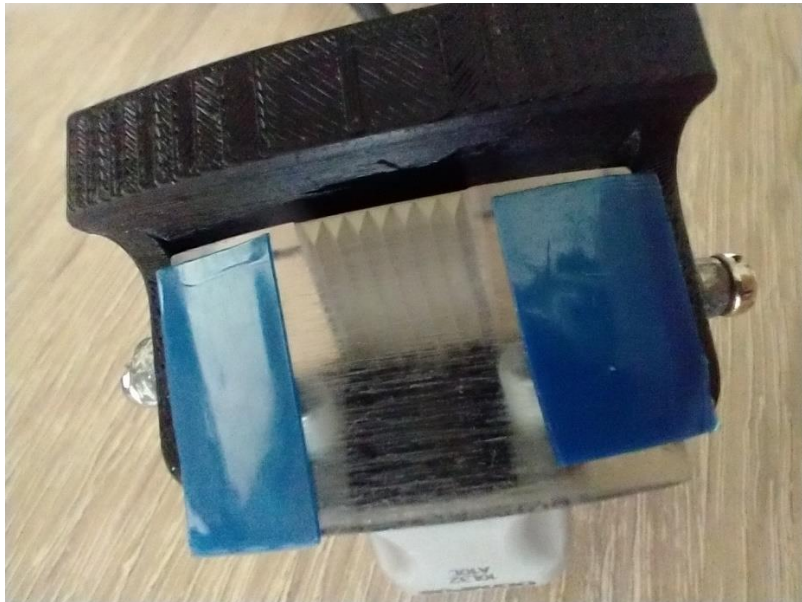
Figure 3-9 Tapes are applied on the side of the wedge to mitigate the wobbling effect and thus to improve consistency.
