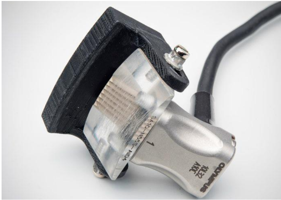
Figure 3-2 The linear PA transducer, wedge and guide used for the inspection.
