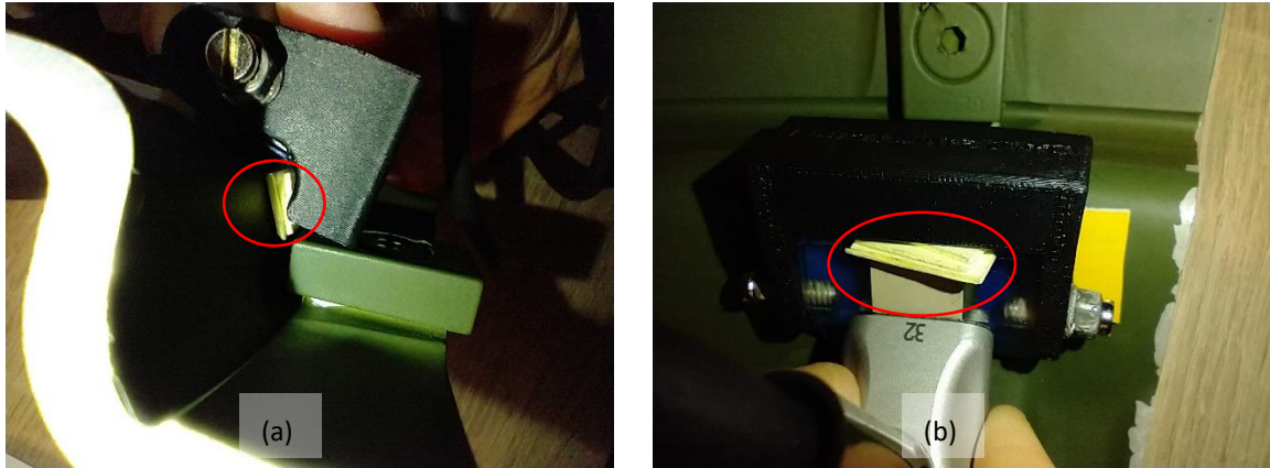
Figure 3-7 Layers of paper put between the guide to adjust the lateral position of the wedge. (a): Layers of paper added in a way that the wedge is positioned in a forward position (+) with respect to the default position. (b): Layers of paper added to move the wedge in a backward position (-) with respect to the default position.
