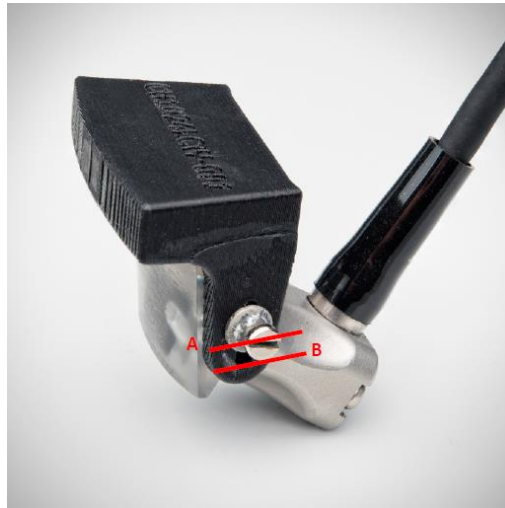
Figure 9-31 The guide on the wedge. It can be either mounted at position A (shown in the figure) or at position B.
