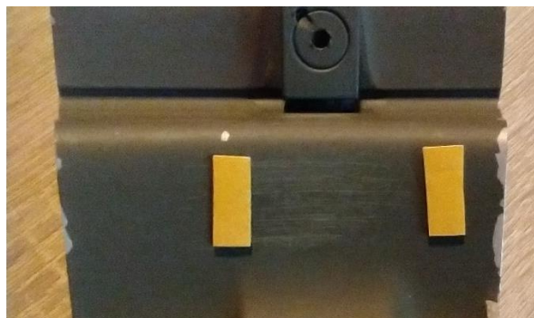
Figure 3-6 Tape is attached on the test specimen to assist the placement of the wedge in the radial direction.
