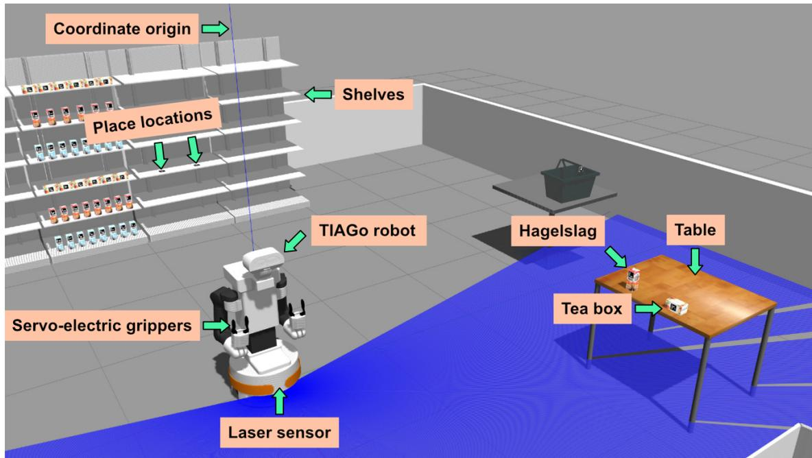
**Figure 5-1:** Figure displaying the lab environment where the robot TIAGo++ is operating. It displays both stocked and empty shelves, with two ArUco markers marking the place locations of the objects. TIAGo++ in this depiction has dual servo-electric grippers, and lasers are displayed in blue. The table has two products with different properties on top. These products are Hagelslag (Dutch chocolate sprinkles) and a tea box.
