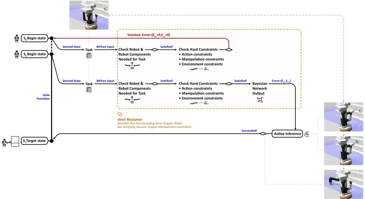
**Figure 5-6:** Experimental case with a picking task. This case demonstrates the reasoning capabilities of the Airet framework, applied to the real TIAGO++ robot in a retail store environment. The hard constraint pertaining to the object width is not satisfied by the aero-electric gripper but is satisfied by the Vacuum gripper, together with other constraints like payload. The picking action with the vacuum gripper is executed, resulting in successful task completion.
