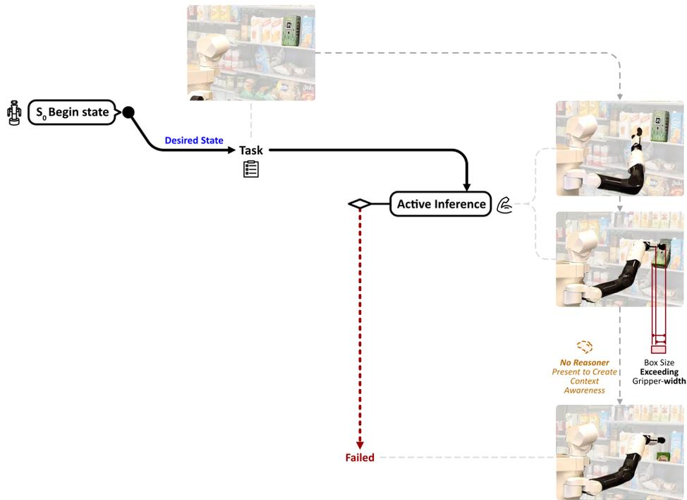
**Figure 5-4:** Experimental case on the real robot with a picking task, no reasoner being present, and the task being ill-defined. It demonstrates task failure due to a lack of context-awareness, manifested in the tipping of the product.
