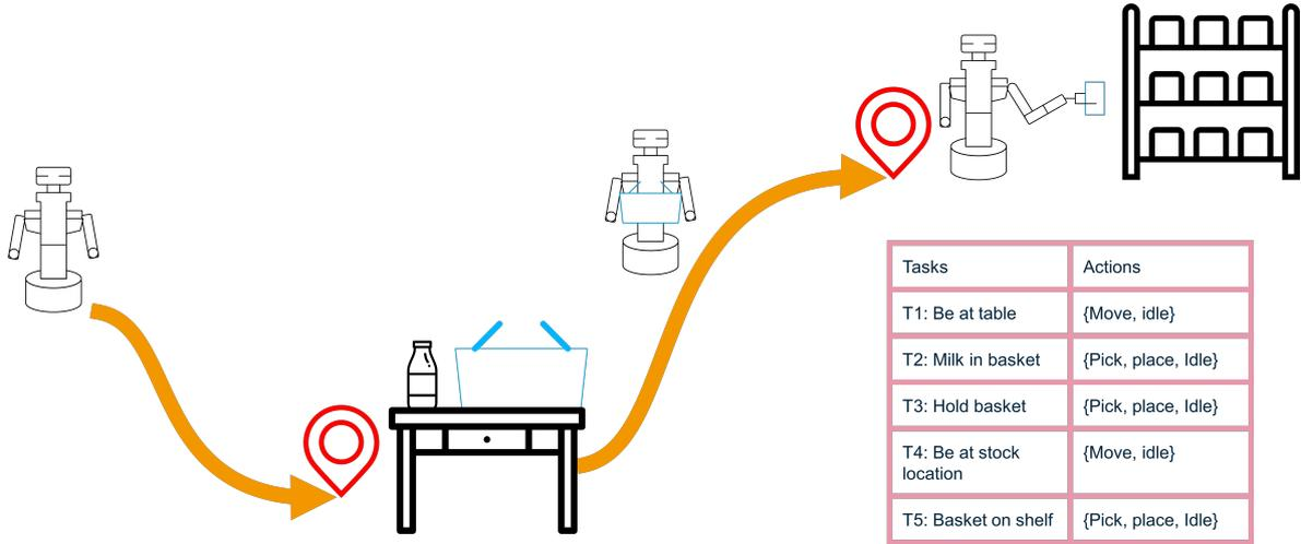
**Figure 3-3:** Example plan generated through the reactive action planning framework using Active Inference of Pezzato et al. [72]. The tasks are formulated as desire  $C$  and selected according to the plan created by an adapted behaviour tree.
