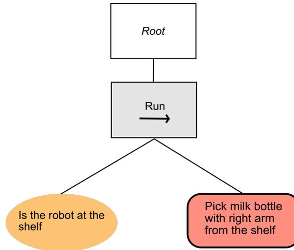
**Figure 3-1:** Simple behaviour tree example depicting an action, condition, sequence and root node. The action node (red square) executes a picking action dependent on a shelf location. The condition node specifies this location as a criterion for the picking action to be executed. If this condition is not met, the pick action is not executed, and failure is returned to the sequence node.
