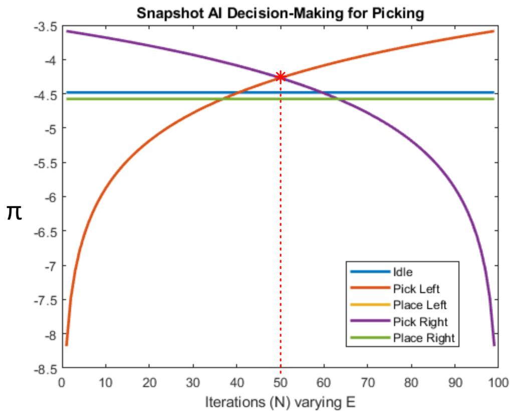
**Figure 4-6:** Snapshot of decision-making through Active Inference for picking. The prior over plans for picking with the left gripper are modelled to increase during each iteration with a value of 0.01 leading up to maximum likelihood of success (value 1). The right gripper is modelled the opposite, starting at the maximum likelihood of success and decreasing during each iteration until it comes close to zero. The x-axis divided by 100 equals the prior over plans.
