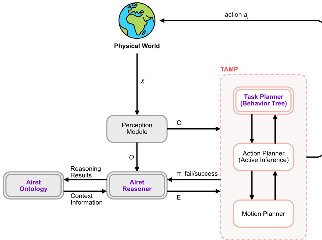
**Figure 4-4:** Figure displaying the cognitive architecture of the Airet framework.  $\Xi$  are the observations of the real environment,  $O$  are the observations translated to an understandable manner for the robotic agent.  $E$  is the prior over plan and  $a_t$  are the actions.
