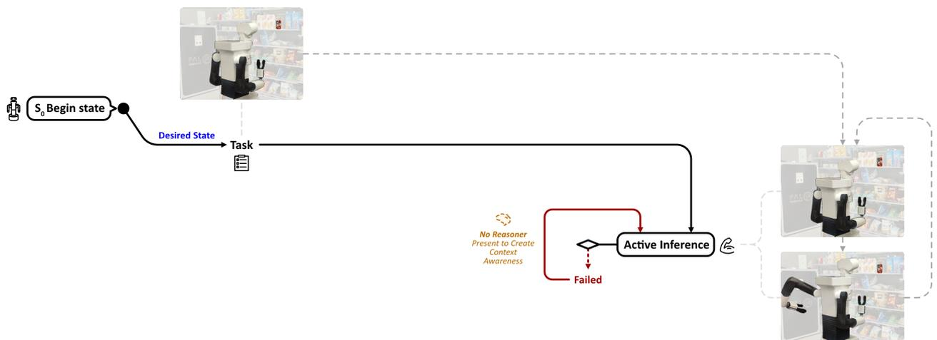
**Figure 5-9:** Experimental case on the real robot demonstrating the repeated picking task failure when dealing with component failure. This is because the decision-making using Active Inference with the task planning framework [74] selects actions that minimise uncertainty in a fixed order. Context-awareness could distinguish between these actions to prefer functioning controllers, based on reasoning on failure.
