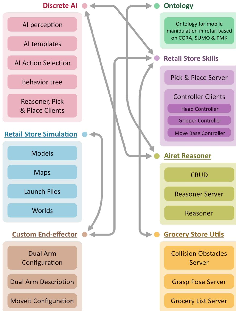
**Figure 5-3:** This figure provides the System Overview of the packages, the ones fully developed in green (the ontology in apple green and reasoner in olive green) and the other packages modified and extended for context-aware mobile manipulation with Active Inference in a retail environment. Communication between modules of packages is facilitated through the ROS platform.
