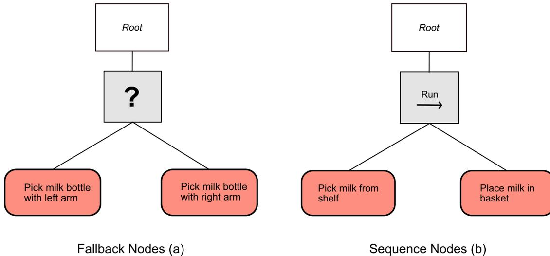
**Figure 3-2:** Simple behaviour trees depicting fallback nodes (a) and sequence nodes (b). (a) place action is only executed when pick action succeeds. (b) If picking with left arm fails, then picking with right arm will be attempted. When no failure occurs this node is skipped.
