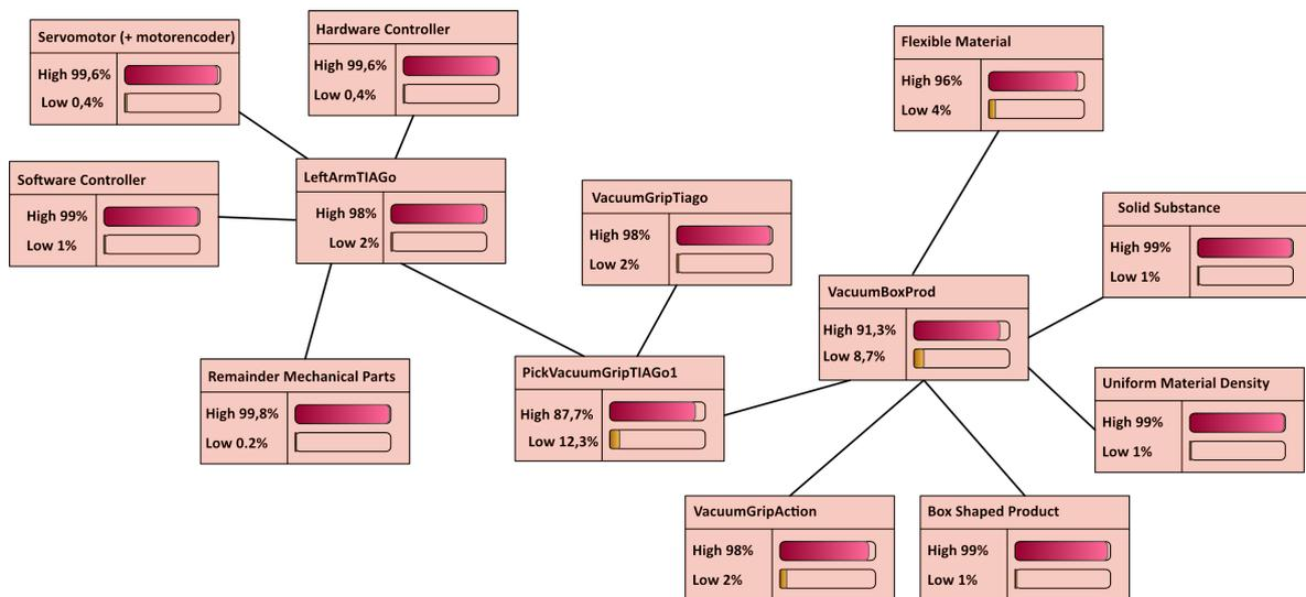
**Figure 5-7:** Bayesian Network with priors over plans demonstrating the factors influencing the decision making for picking a box-shaped product with a vacuum gripper attached to the left arm. The Bayesian Network is populated through the ontology. Fault detection & isolation methods are assumed to provide information on the failed component.
