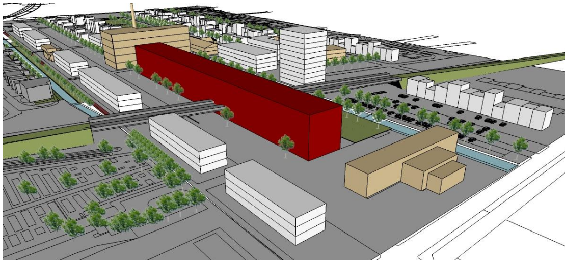
The building mass of the station building (red) in its urban context. White volumes are new volumes, brown volumes are existing (industrial) buildings
