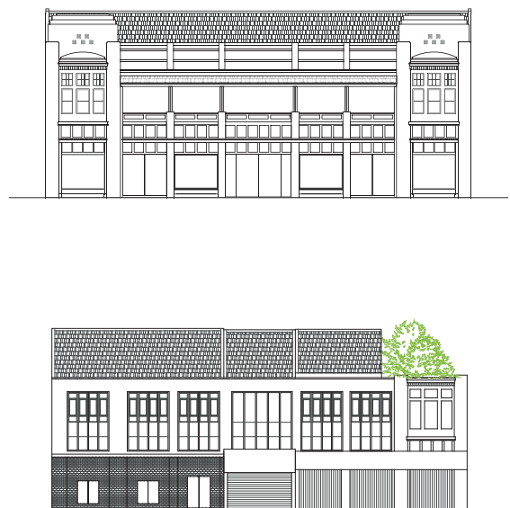
Figure 3. The drawing above illustrates the original facade and the drawing below illustrates the current situation
