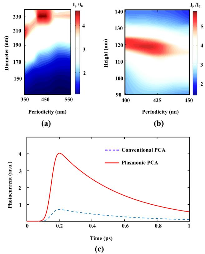
Fig. 2. (a) Distribution of plasmonic PCA photocurrent as a function of nanodisks periodicity (P) and Diameter (D) at nanodisk height of  $H = 100$  nm (b) Distribution of plasmonic PCA photocurrent as a function of nanodisks periodicity (P) and height (H) at nanograting width of  $D = 230$  nm (c) Photocurrent of plasmonic PCA in comparison with conventional PCA.
