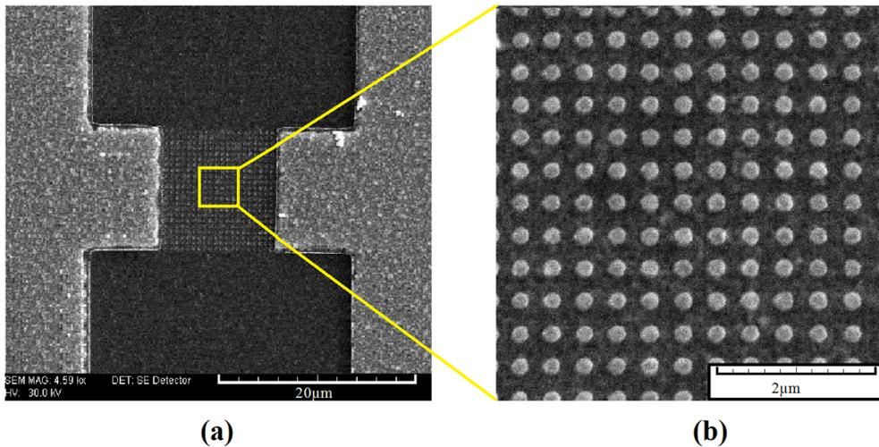
Fig. 5. (a) SEM image of the dipole PCA with the nanodisk array (b) a magnified image of the Ti/Au nanodisk array.
