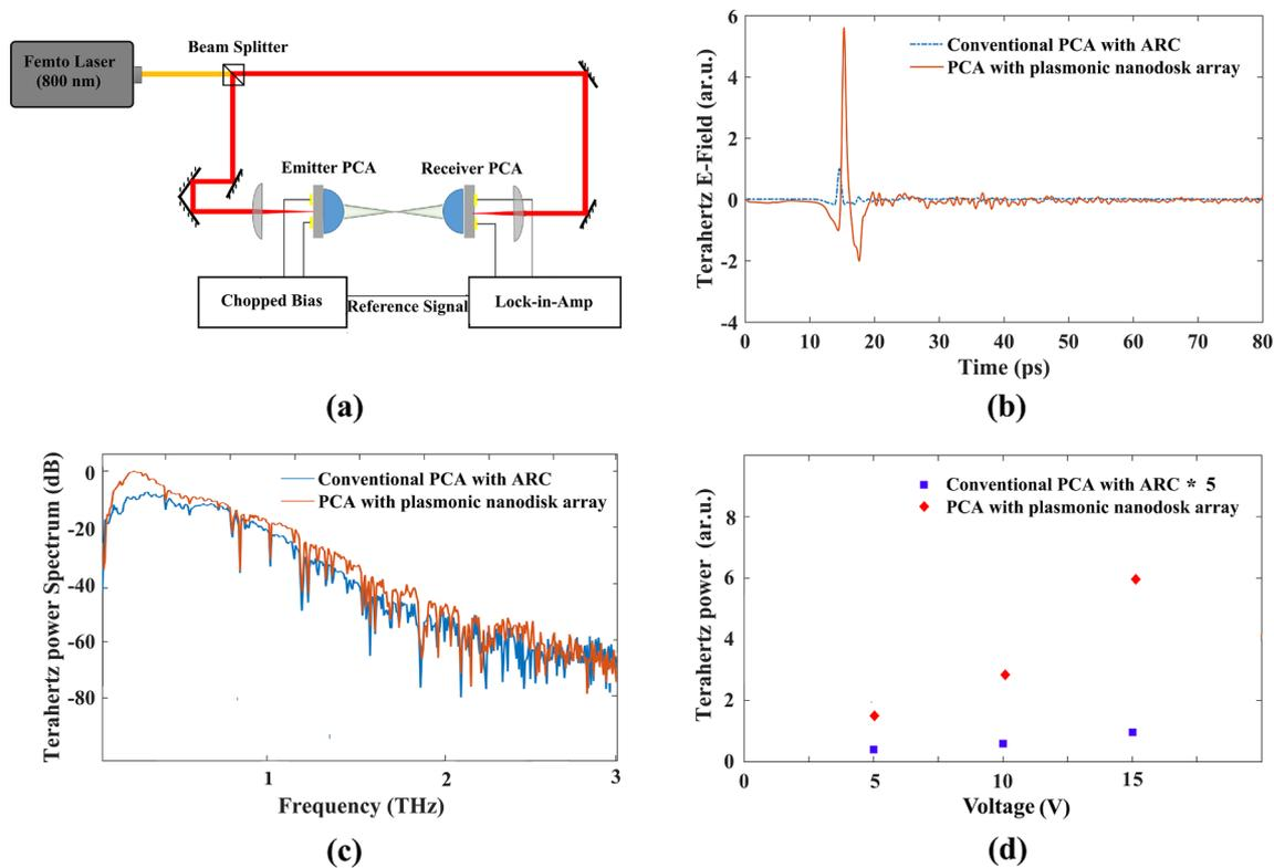
Fig. 6. (a) The schematic of the experimental setup for measuring THz generation using an 800 nm fs laser (b) THz E-Field as a function of time and (c) THz radiation power comparison of a PCA with ARC and a similar PCA with nanoplasmonic structure and (d) Power trends vs bias for PCA with optimized plasmonic structure (red) and conventional PCA with ARC (blue). (For interpretation of the references to colour in this figure legend, the reader is referred to the web version of this article.)
