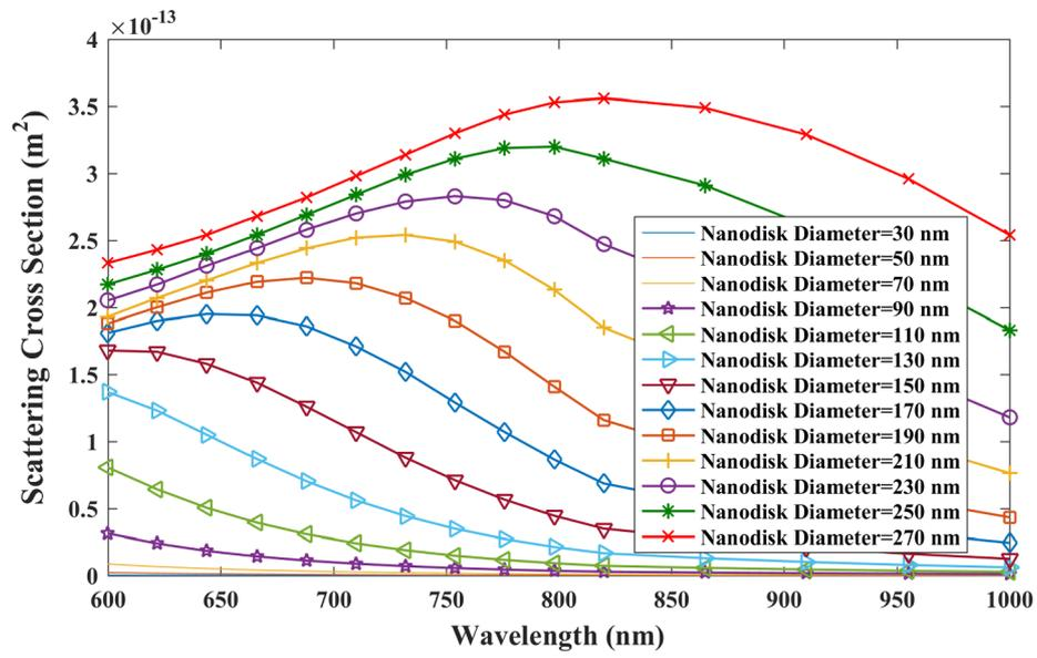
Fig. 3. Scattering cross section of nanodisks as a function of wavelength for different diameter.
