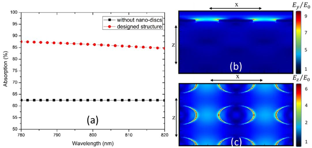
Fig. 4. (a) The absorption efficiency of the antenna with and without nanodisk, (b) side view of the E-field distribution, and (c) top view of the E-field distribution.
