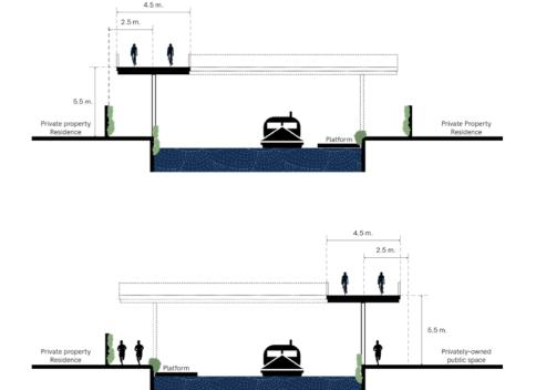
Figure 8.16. Typical sections of the proposed path
