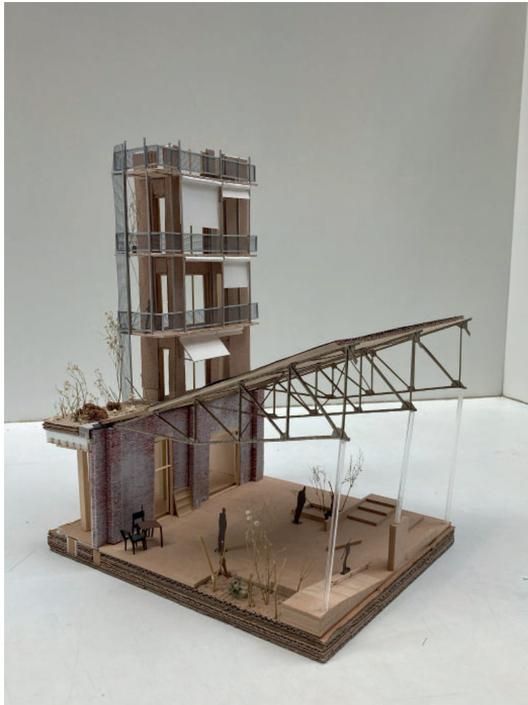
1:33 fragment model. The model fragment is of the crossingpoint between three building parts: the passage, the housing and the retail. To show the different types of construction and materiality.
