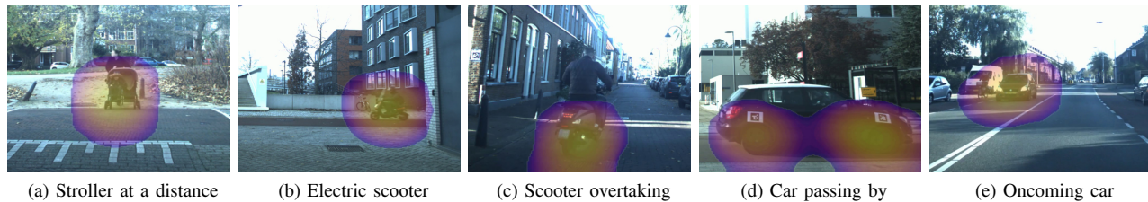
Fig. 4. Qualitative examples of 2D Direction-of-Arrival estimation overlaid on the camera image (zoomed). (a): Stroller wheels are picked up even at a distance. (b), (c): Both conventional and more quiet electric scooters are detected. (d): The loudest sound of a passing vehicle is typically the road contact of the individual tires. (e): Even when the ego-vehicle drives at \sim 30 km/h, oncoming moving vehicles are still registered as salient sound sources.
