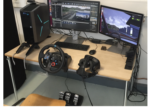
Fig. 1: The HMD-based VR driving simulator setup.
