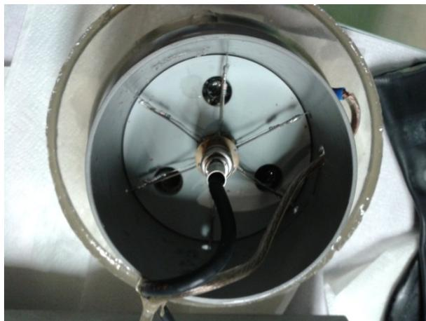
(b) Backside of the electrode, impedance Z (6 impedances of 300 Ohm in parallel connected with plane electrode) and transmission line connected with the impedance Z.
