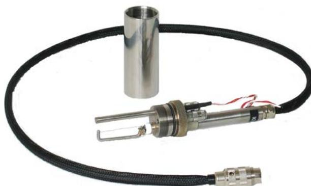
Figure 5.3 Lambda sensor head.
