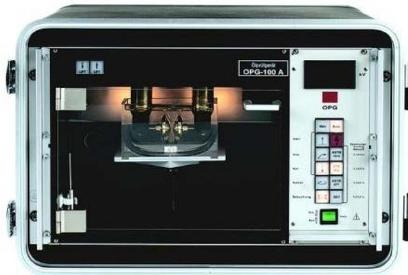
Figure 3.1 OPG-100A insulating oil tester.
