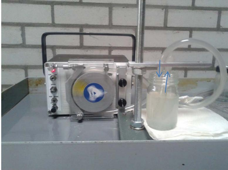
Figure 6.5 Modified test set-up with the tube entering the beaker in the centre.
