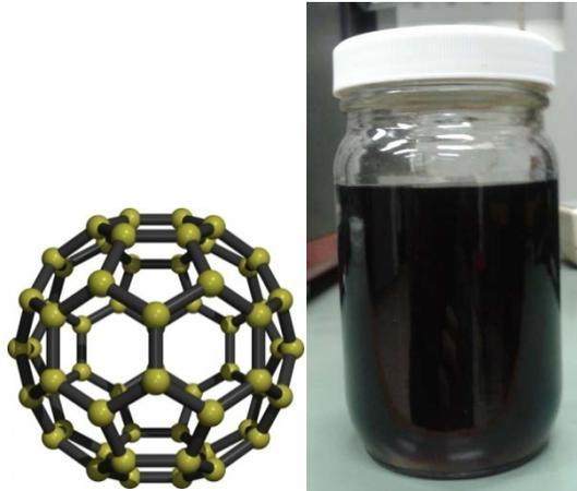
Fig.3.14 molecular structure of fullerene C60, 0.05% fullerene nanofluids.
