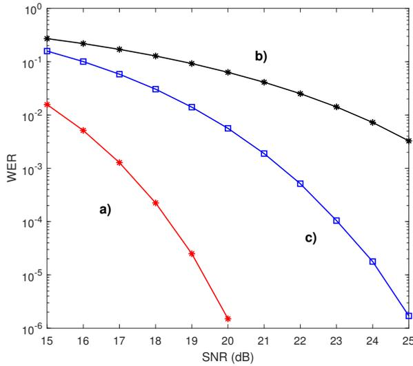
Figure 6.6: Word error rate (WER) for  $n = 7$  and  $q = 2$ , a) without channel mismatch, b) with channel mismatch  $a = 1.07$ ,  $b = 0.07$ , and  $c = 0.04$  both using minimum Euclidean distance detection, and as a comparison c) for the proposed scheme that MPD is used with a difference operator.
