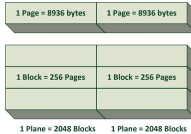
Figure 1.1: Structure of storage array inside Flash.
