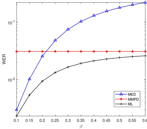
Figure 3.8: Simulated word error rate (WER) versus the standard deviation of the offset of MED, MMPD, and ML detectors for (3,2) parity check code when the standard deviation of the noise  $\sigma = 0.2$ .
