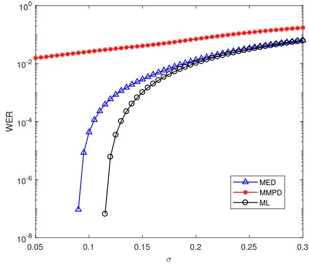
Figure 4.1: WER versus the standard deviation  $\sigma$  of the uniform noise for  $S^*$  in combination with MED, MMPD, and ML decoders, when the standard deviations of the uniform offsets are  $\beta_0 = 0.2$ ,  $\beta_1 = 0.15$ .
