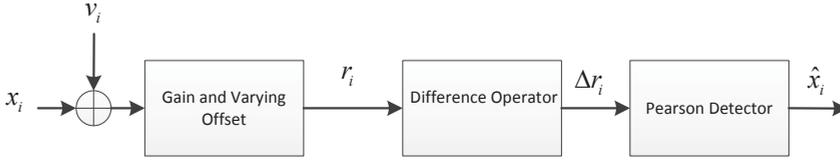
Figure 6.1: MPD detection using a difference operator.
