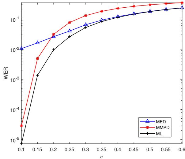
Figure 3.7: Simulated word error rate (WER) versus the standard deviation of the noise of MED, MMPD, and ML detectors for (3,2) parity check code when the standard deviation of the offset  $\beta = 0.2$ .
