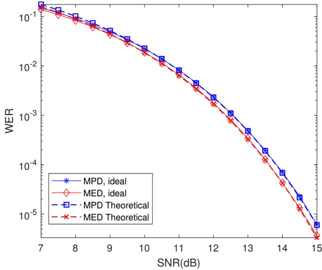
Figure 2.6: Theoretical upper bounds and simulated word error rate (WER) as a function of signal to noise ratio (SNR) for the modified (7,4,3) Hamming code. The theoretical performances are computed by upper bounds (2.22) and (2.37), and simulation curves are obtained for the ideally matched channels ( $a = 1, b = 0$ ) with only Gaussian noise.
