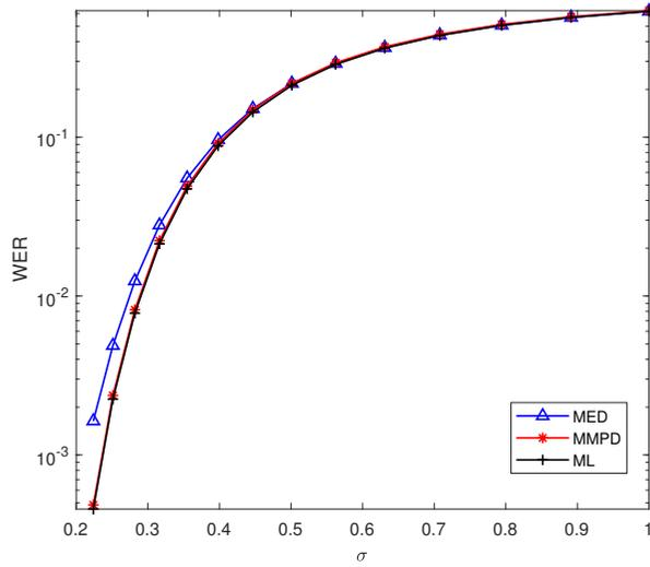
Figure 3.9: Simulated word error rate (WER) versus the standard deviation of the noise of MED, MMPD, and ML detectors for modified (7,4,3) Hamming code when the standard deviation of the offset  $\beta = 0.2$ .
