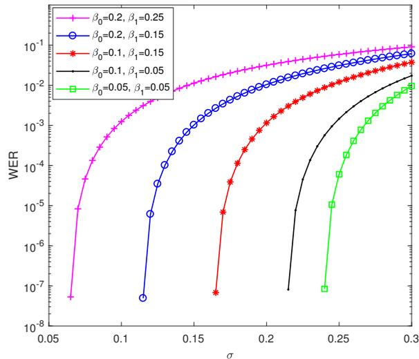
Figure 4.2: WER versus the standard deviation  $\sigma$  of the uniform noise for  $S^*$  in combination with ML decoding, with different values of the uniform offset standard deviations  $\beta_0$ ,  $\beta_1$ .
