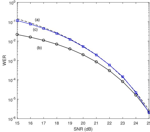
Figure 6.5: Word error rate (WER) as a function of the signal-to-noise ratio ( $\text{SNR} = -20 \log_{10} \sigma$ ), for  $n = 7$  and  $q = 2$  computed using upper bound (6.37), curve (a), and by using the approximation (6.38), curve (b). The square marked line (c) shows simulated results of the proposed scheme with channel parameters  $a = 1.07$ ,  $b = 0.07$ , and  $c = 0.04$ .
