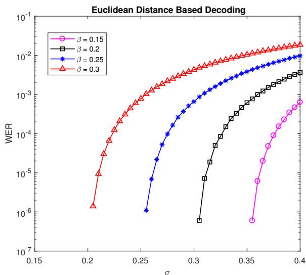
Figure 3.1: Simulated WER of Euclidean distance based decoding for codebook  $S^*$  on channels with uniform noise  $v_i \sim \mathcal{U}(-\sigma, \sigma)$  and uniform offset  $b \sim \mathcal{U}(-\beta, \beta)$ .
