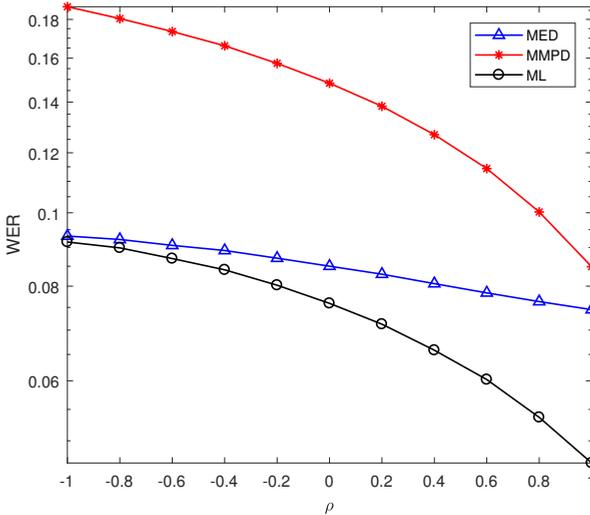
Figure 4.5: Simulated word error rate (WER) versus  $\rho$  of  $S^*$  for channels with Gaussian noise and signal dependent offsets, that standard deviations  $\beta_0 = 0.2$ ,  $\beta_1 = 0.3$ , and signal to noise ratio is 12 dB.
