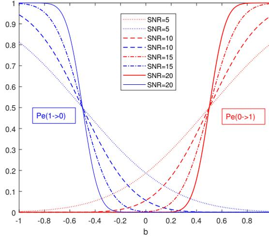
Figure 2.2: Probabilities of  $0 \rightarrow 1$  and  $1 \rightarrow 0$  errors as a function of SNR assuming different values of the offset  $b$ , where  $Pe(0 \rightarrow 1)$  and  $Pe(1 \rightarrow 0)$  correspond to  $\Pr(r_i \geq V_m | x_i = 0)$  and  $\Pr(r_i < V_m | x_i = 1)$ , respectively.
