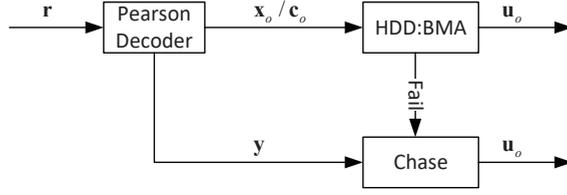
Figure 3.12: Block diagram of the decoding algorithm.
