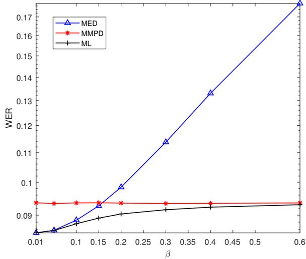
Figure 3.10: Simulated word error rate (WER) versus the standard deviation of the offset of MED, MMPD, and ML detectors for modified (7,4,3) Hamming code when the standard deviation of the noise  $\sigma = 0.4$ .
