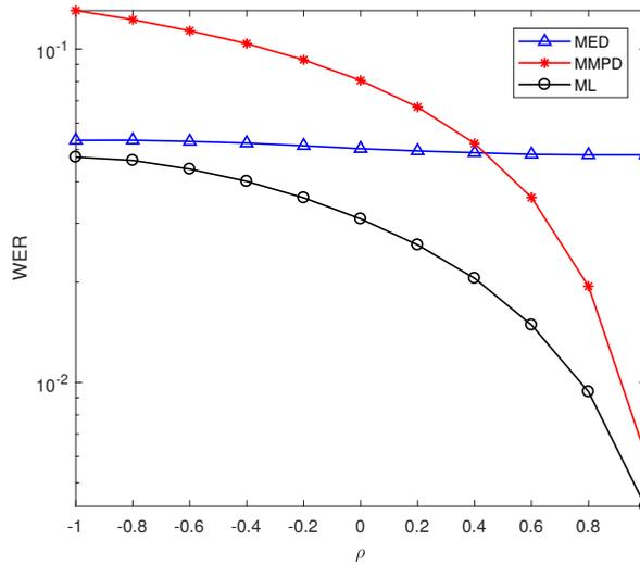
Figure 4.6: Simulated word error rate (WER) versus  $\rho$  of  $S^*$  for channels with Gaussian noise and signal dependent offsets, that have standard deviations  $\beta_0 = 0.2$ ,  $\beta_1 = 0.3$ , and signal to noise ratio is 17 dB.
