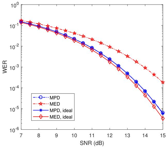
Figure 2.7: Simulated word error rate (WER) as a function of signal to noise ratio (SNR) for the modified (7,4,3) Hamming code in the ideally matched case ( $a = 1, b = 0$ ) and the situation with  $a = 1.1$  and  $b = 0.3$ .
