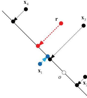
Figure 2.5: Graphic illustration of the minimum modified Pearson distance based detection of four codewords.
