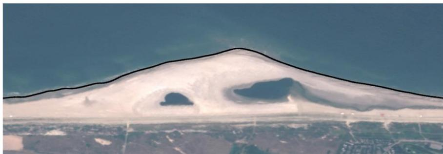
Figure 5 Satellite image acquired by the Sentinel 2 satellite acquired on 12-03-2015 10:33:27 (GMT) for the Sand Motor study site. The derived SDS is plotted in black. From Hagenaaers et al. (2018).
