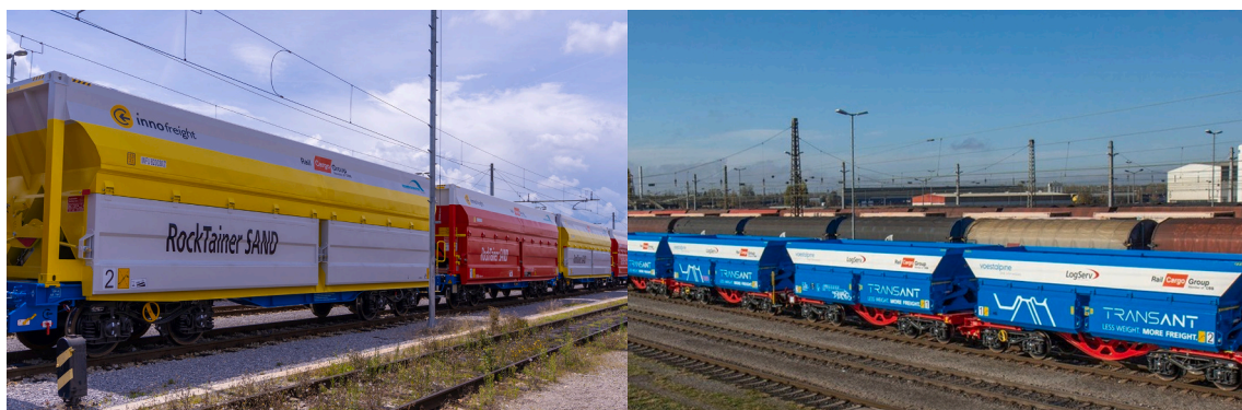
Fig. 1. InnoWaggon RockTainer SAND by Innofreight (left) (Innofreight, 2026) and TransANT hopper wagon (right) (TransANT, 2026)
