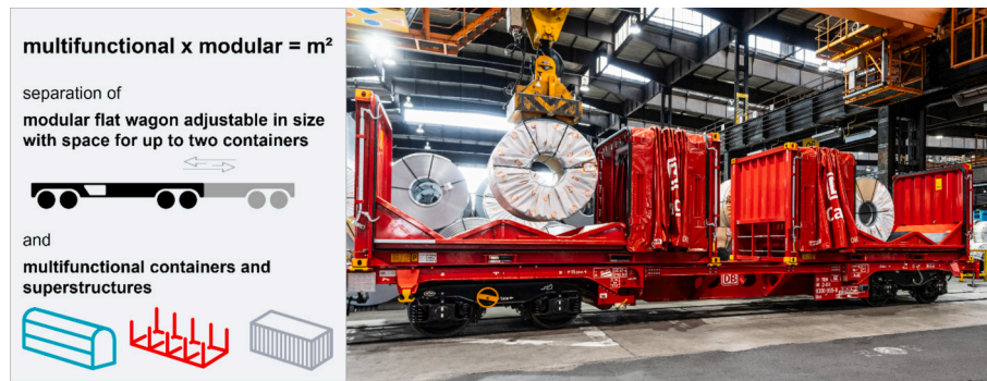
Fig. 2. The m^2 freight wagon by DB Cargo (Author's work, photo by DB Cargo).
