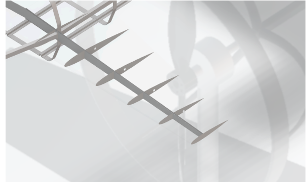
Figure 9.9: Internal Structural Layout of the Canard Assembly
