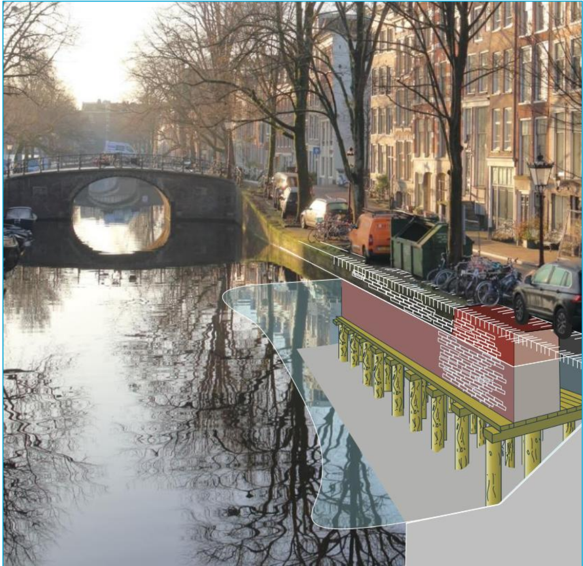
Figure 2 - Cutaway drawing of historical quay wall structure at Reguliersgracht (Hemel, 2023)
