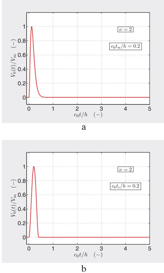
Fig. 2. Excitation pulse shape. (a) Unipolar PE pulse; (b) unipolar WP pulse.
