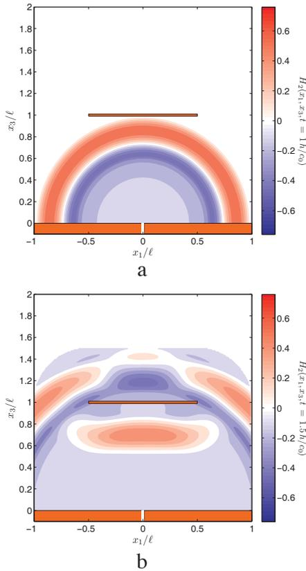
Fig. 4. The magnetic-field spatial distribution observed at (a)  $c_0t = 1.00h$  and (b)  $c_0t = 1.50h$  – WP excitation.
