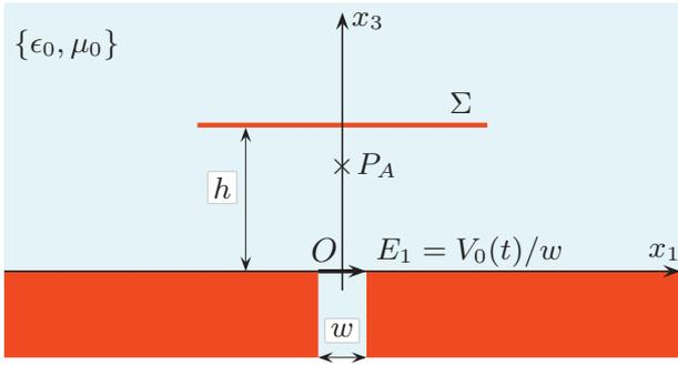
Fig. 1. A Fabry-Perot slot-excited resonator antenna.
