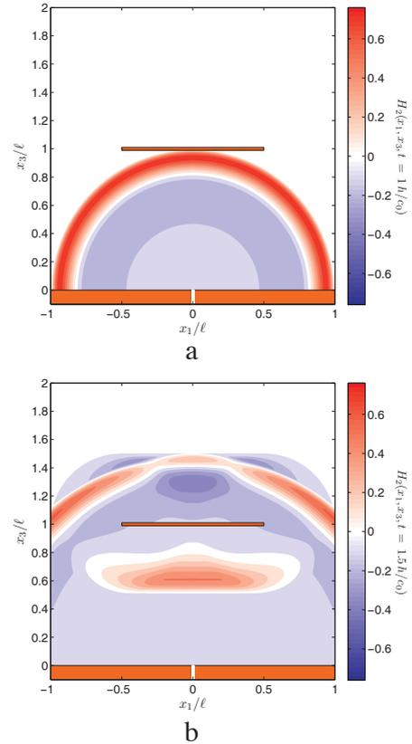
Fig. 3. The magnetic-field spatial distribution observed at (a)  $c_0 t = 1.00h$  and (b)  $c_0 t = 1.50h$  – PE excitation.
