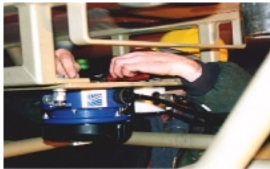
Fig. 3.4 Attaching the ADCP in the iron cage
