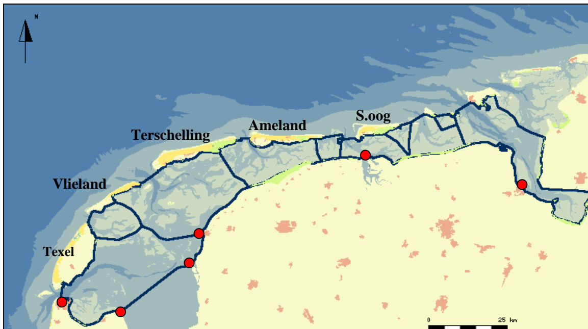
Fig. 1.1 The tidal basins of the Dutch Wadden Sea. The black lines represent the watersheds between the basins. The red dots represent the sluices, which regularly supply fresh water into the Wadden Sea.
