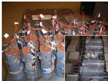
Fig.1 The reinforced concrete specimens (red mud and BFS containing mixtures) after casting (before de-moulding).
