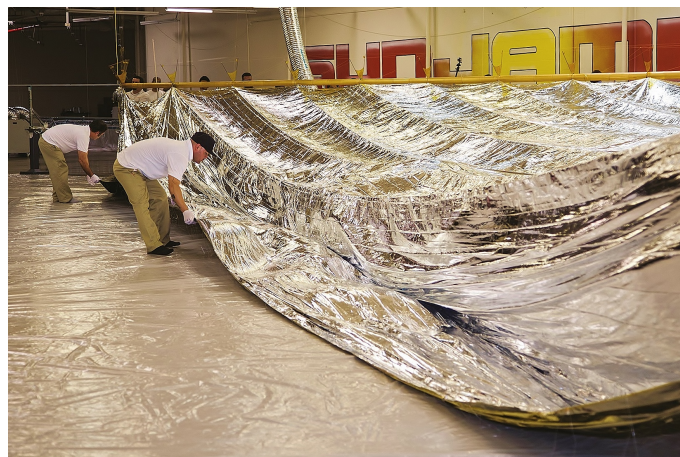
Figure 2.2: Engineers extend one of the four quadrants of Sunjammer's solar sail [Space.com, 2013b].
