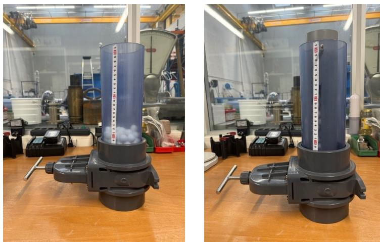
**Figure C.1:** L: Nodule dispenser 55 % and 10cm height, R: Nodule dispenser 26% and height of 20 cm
