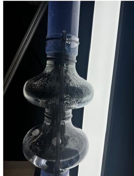
**(b)** View from the right side showing solids retained.**Figure 5.1:** Comparison of Left and Right Views: Test Results with 30 mm Solid Showing Solids Retained at Different Locations.
