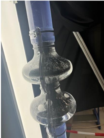
**(a)** View from the left side showing solids retained.
