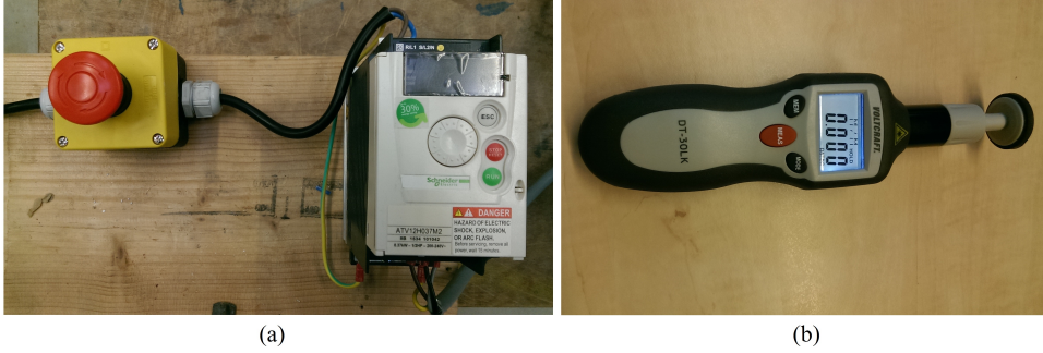
Figure 6.4: Controlling and measuring the speed of belt conveyor: a) Variable-frequency drive controller, b) Voltcraft speedometer.
