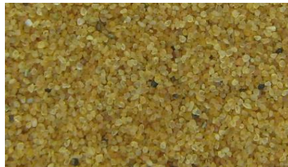
Figure 6.7: The shape of quartz sand grains.
