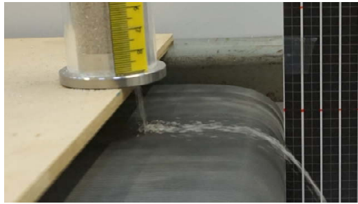
Figure 6.8: Position of the sand feeder on the belt conveyor set-up.
