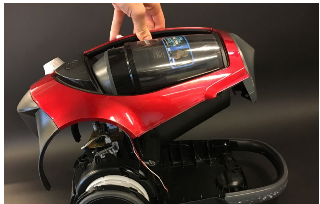
Single step disassembly of the upper clump, composed by all the plastic casings.
