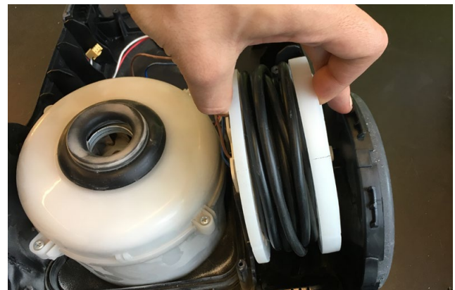
Independent disassembly of cord-winder and motor assy
