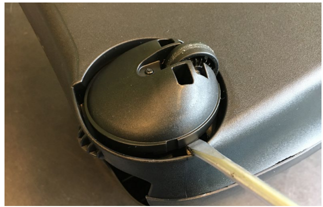
Easy external disassembly of the wheels, using a spudger
