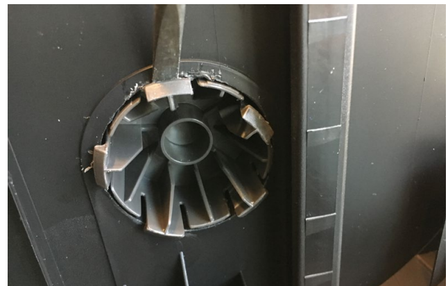
Wheel fastening system in the FC9569, composed by robust snap fits which have to be broken in order to disassemble the wheel
