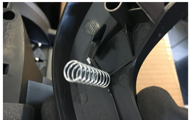
Broken hidden snap fits while trying to disassemble the part
