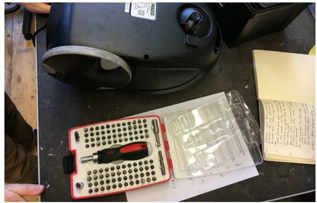
Special kit of uncommon tools used by the repairer
