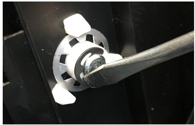
Disassembly of the wheels on the FC9934 and FC8924, removing a metal ring which fastens the wheel bearing
