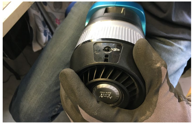
Repairer showing a small insert which is always lost during the disassembly
