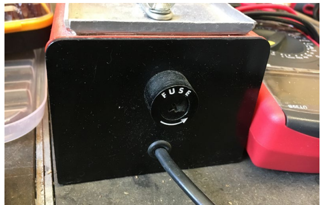
Example of external product fuse, used by the repairer to explain the importance of accessible priority components
