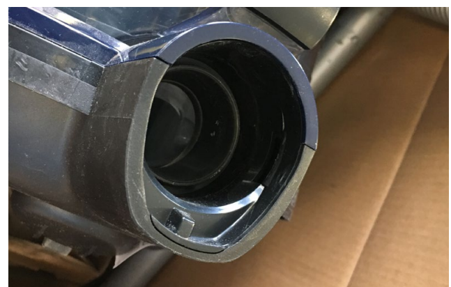
Example of hidden assembly difficult to disassemble
