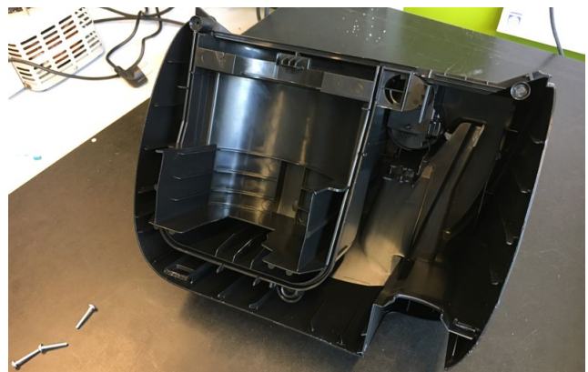
Big plastic clump, grouping together rear housing and motor housing lid, removable together in one step.
