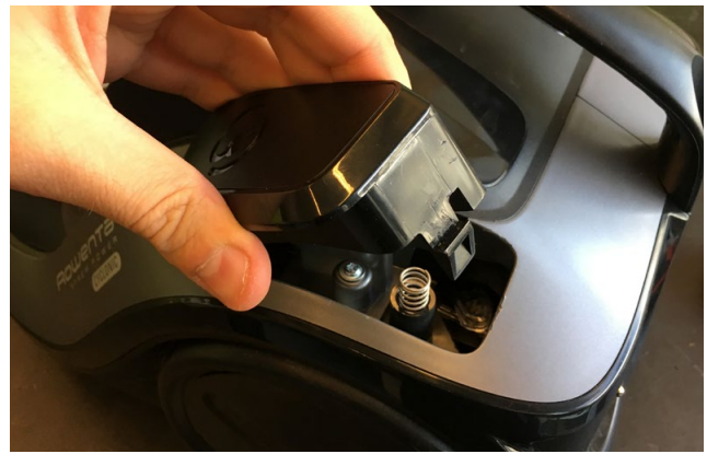
Complex disassembly of buttons, necessary to reach hidden screws
