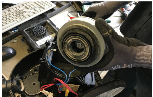
Repairer showing and explaining main causes of motor breakage
