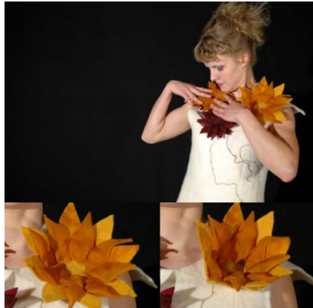
FIGURE 2.28: KUKKIA DRESS BY XS LABS WITH NITINOL WIRE STITCHED ONTO THE PETALS FOR OPENING AND CLOSING OF THE FLOWER (BERZOWSKA & COELHO, 2005)
