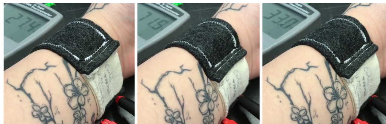
FIGURE 5.30: CURLED U SHAPE 16CM PROTOTYPE WITH 1MM DIAMETER SMA WIRE TESTED ON MY WRIST. [FROM LEFT TO RIGHT] BEFORE ACTIVATION (27.4°C), AUSTENITE STATE (71.5°C), AND COOLED AFTER ACTIVATION (33.0°C)
