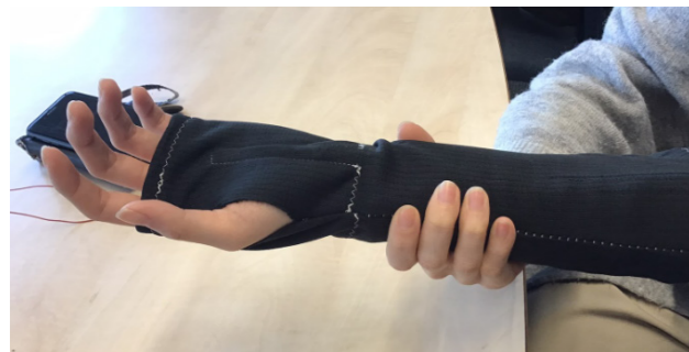
FIGURE 6.31: A PARTICIPANT MASSAGING SERENISLEEVE WHILE IT WAS COOL DOWN TO CONFORM THE SMA WIRES TO HER FOREARM SHAPE
