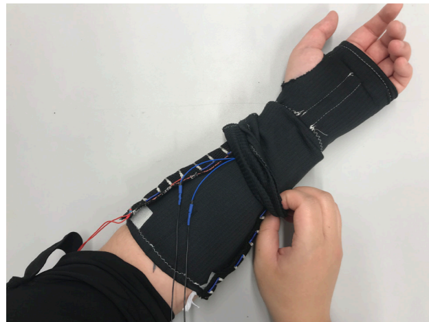
FIGURE 6.16 : THE OUTER LAYER HIDES THE SMA ACTUATOR AND THE FSR SENSOR WIRES, SO THE OVERALL WEARABLE IS DISCREET, AND THE ELECTRONIC COMPONENTS ARE PROTECTED FROM THE ENVIRONMENT.
