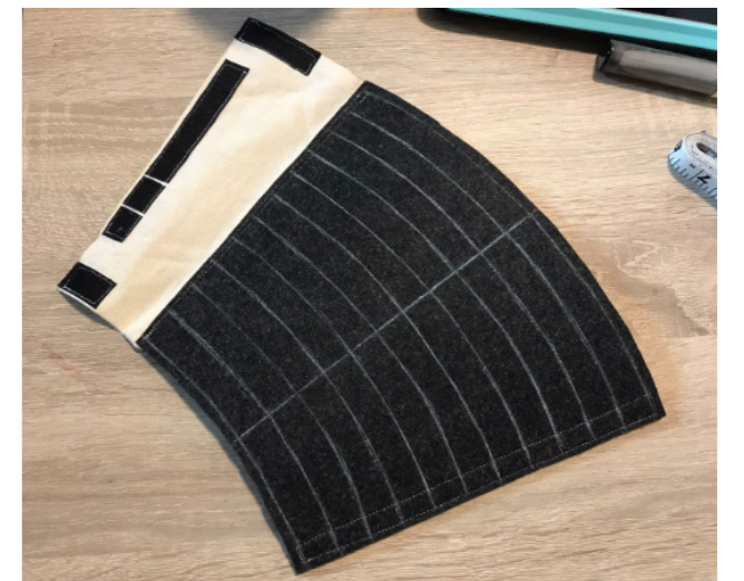
FIGURE 6.2: FELT AND MUSLIN FABRIC SLEEVE WITH APPROXIMATE LOCATIONS FOR THE SMA WIRES DRAWN WITH WHITE CAULK
