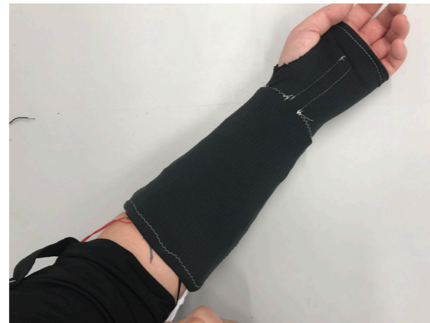
FIGURE 6.17 : THE OUTER LAYER ALSO HAS AN ELASTIC CORD THAT CAN BE USED TO TIGHTEN AROUND THE FOREARM.
