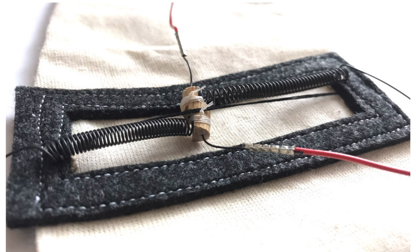
FIGURE 5.9: STROKING ACTUATOR PROTOTYPE WITH TWO M4 SMA SPRINGS IN ANTAGONISTIC DIRECTIONS CONNECTED THROUGH A WOODEN END-EFFECTOR
