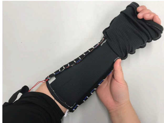
FIGURE 6.14 : 3D MESH SMA ACTUATOR INSERT AFFIXES TO THE INNER LAYER OF THE SLEEVE COVER WITH VELCRO STRIPS. THE INNER LAYER ALSO ACTS AS A MOISTURE WICKING FABRIC BETWEEN THE ACTUATOR INSERT AND THE USER'S SKIN.
