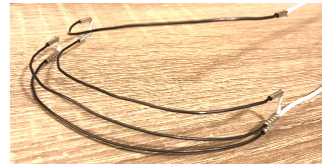
FIGURE 5.39: FOUR HEART SHAPED TRAINED SMA WIRES STRAIGHTENED OUT AND CONNECTED USING ELECTRICAL CRIMPS AND SOLID CORE ELECTRICAL WIRES
