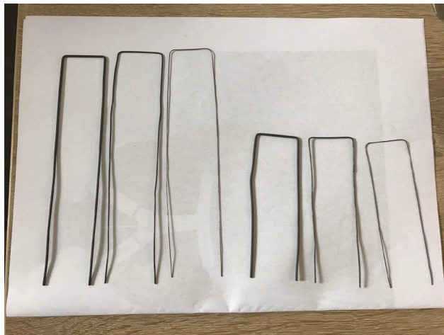
FIGURE 5.17: DIFFERENT DIAMETER “STRAIGHT” SMA WIRES FORMED AND TRAINED INTO U SHAPES FOR ELECTRICAL CONNECTIVITY
