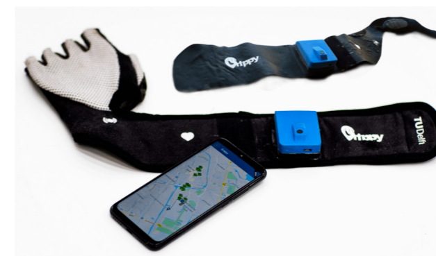
FIGURE 2.3: FINAL PROTOTYPE OF GRIPPY, INCLUDING GLOVE AND STRAP SHAPED WEARABLE AND A MOBILE APP. (LI, 2022)
