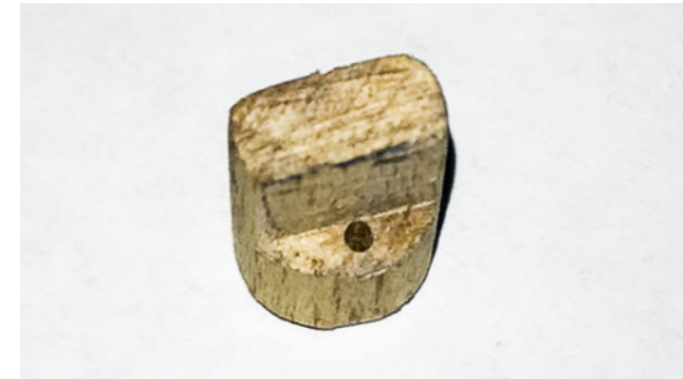
FIGURE 5.7: WOODEN END-EFFECTOR WITH A FLATTENED SIDE AND A SMALL HOLE FOR 0.5MM DIAMETER SMA WIRE TO FIT THROUGH
