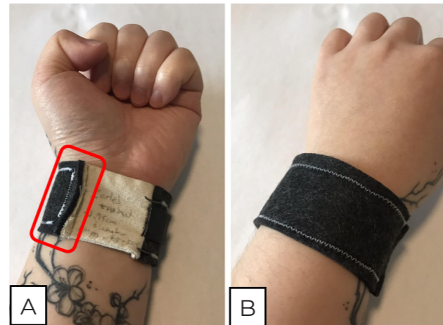
FIGURE 5.35: [A] SHORTER ENDS OF THE SMA EMBEDDED STRAP WITH U SHAPE CONNECTOR BAR HIGHLIGHTED [B] MIDDLE OF THE SMA EMBEDDED STRAP
