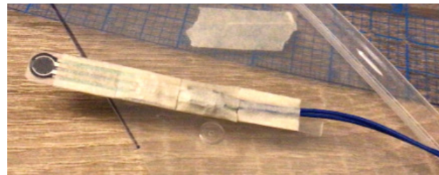
FIGURE 6.8: 5MM DIAMETER FSR SENSOR TAPED TO A 1CM WIDE PLASTIC STRIP CUT FROM A TAKEOUT CONTAINER LID
