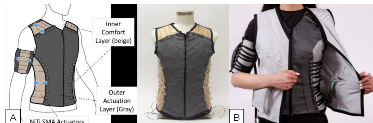
FIGURE 2.14: ARM BAND AND VEST WEARABLE DEVICES WITH SMA ACTUATORS FOR COMPRESSION [A] (FOO ET AL., 2018); [B] (FOO ET AL., 2019)
