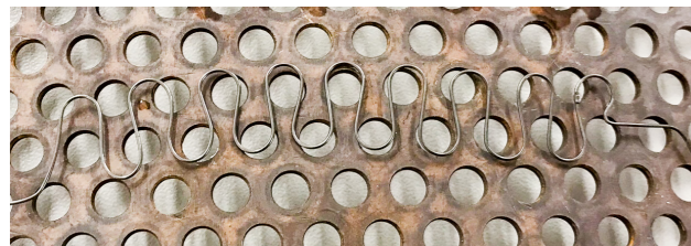
FIGURE 4.4: EXAMPLE OF A ZIGZAG SPRING FORMED USING THE GEOMETRIES OF A PERFORATED METAL SHEET
