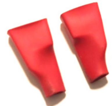
FIGURE 4.12: ELECTRICALLY INSULATING CAPS FOR THE DIGITAL CALIPERS MADE USING HEAT SHRINK TUBING FOR ELECTRICAL WIRES
