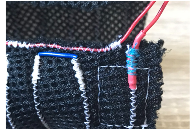
FIGURE 6.33: ELECTRICAL CRIMP CONNECTION POINTS WITH (RED, ON THE RIGHT) AND WITHOUT (BLUE, ON THE LEFT) HEAT SHRINK TUBING
