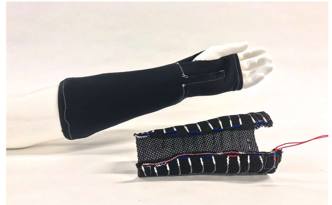
FIGURE 6.11: SERENISLEEVE WITH DOUBLE LAYERED SLEEVE COVER AND 3D MESH SMA ACTUATOR INSERT
