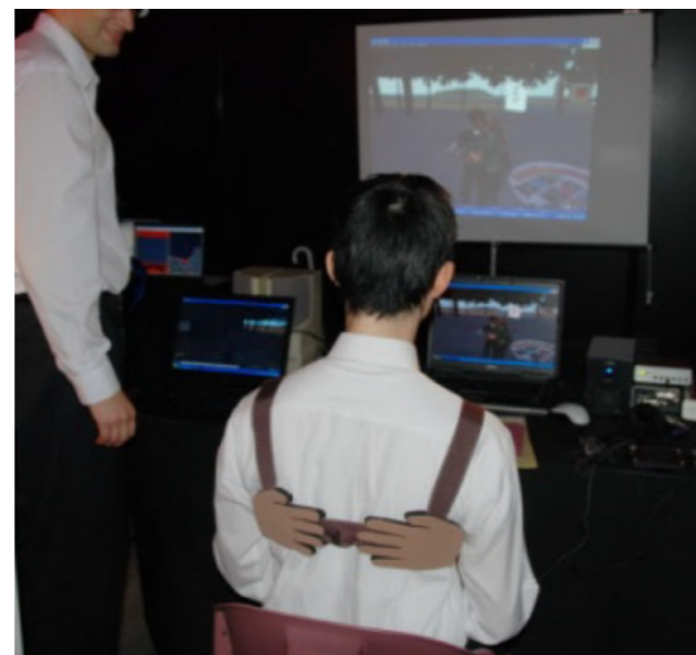
FIGURE 5.2: HAPTIHUG HARNESS PROTOTYPE (TSETSERUKOU, 2010)
