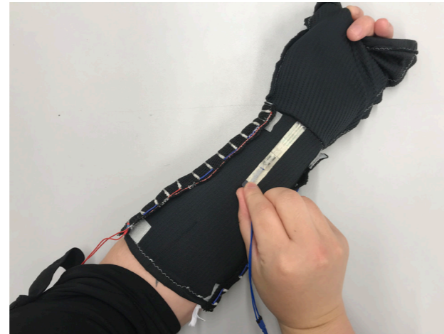
FIGURE 6.15 : 5MM DIAMETER FSR SENSOR ATTACHED TO A STRIP OF FLEXIBLE THIN PLASTIC IS SLIPPED INTO THE POCKET ON THE PALM AREA.
