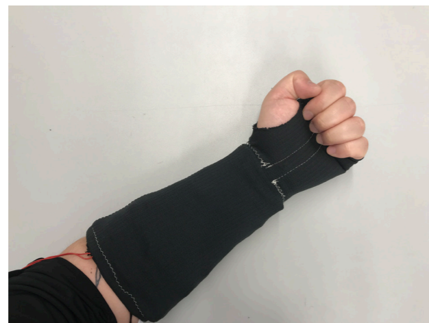
FIGURE 6.18 : SERENISLEEVE IS ACTIVATED BY MAKING A FIST AND HOLDING DOWN THE FSR SENSOR BUTTON FOR A FEW SECONDS.
