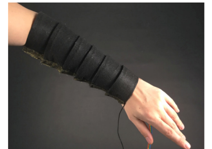
FIGURE 2.15: AFFECTIVE SLEEVE PROTOTYPE WORN ON THE FOREARM (PAPADOPOULOU ET AL., 2019)
