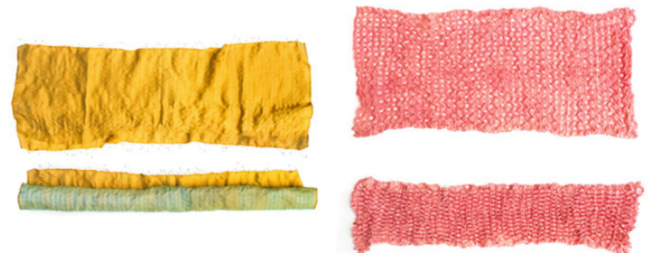
FIGURE 2.27 : SHAPE MEMORY TEXTILE DESIGNED AND CRAFTED BY MARIELLE LEENDERS USING THIN NITINOL WIRES WEAVED INTO OR STITCHED ONTO THE TEXTILE (BENGISU & FERRARA, 2018)
