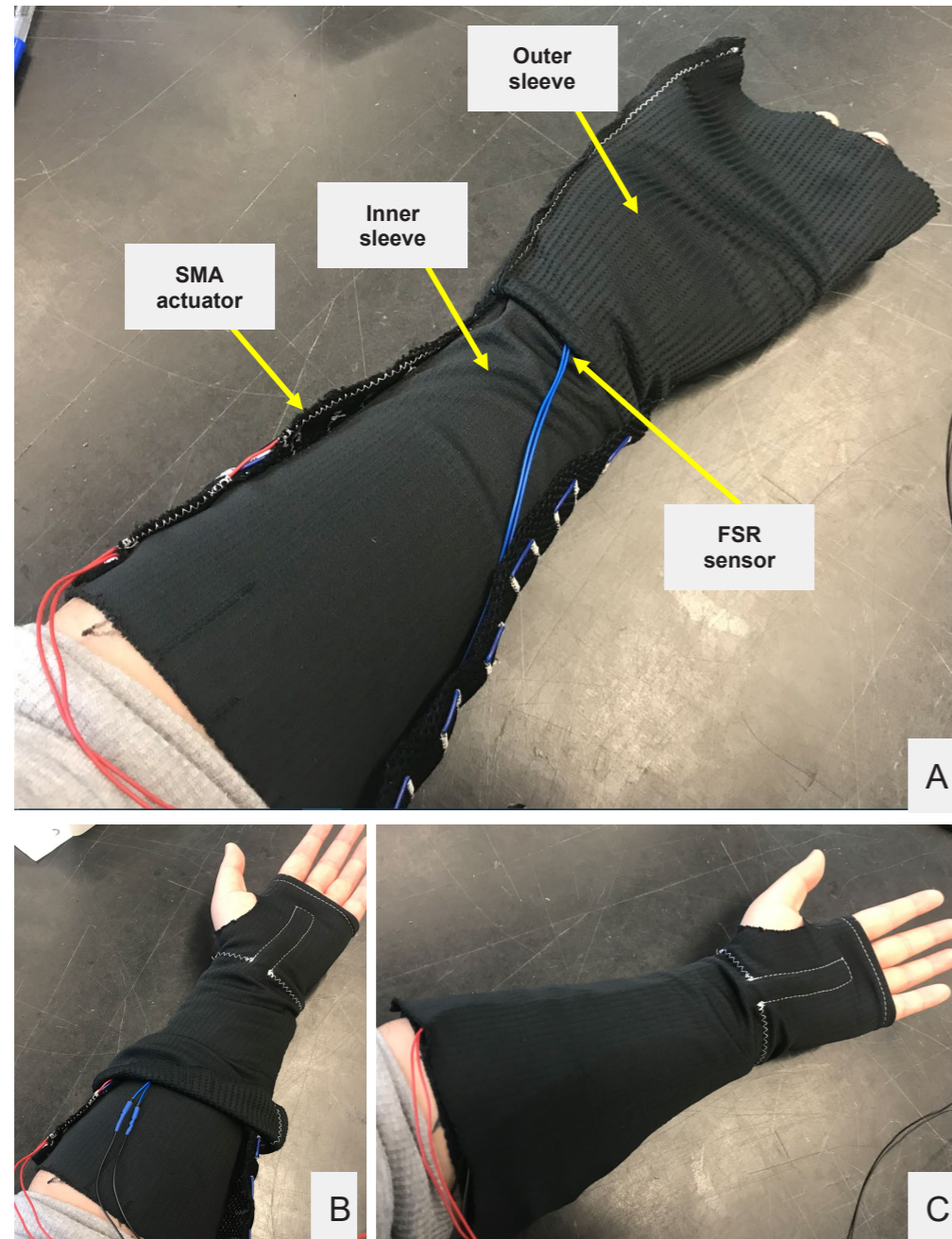
Picture 3: (A) Inner assembly of sleeve, (B) outer sleeve slide over SMA actuator, (C) Fully assembled wearable sleeve device
