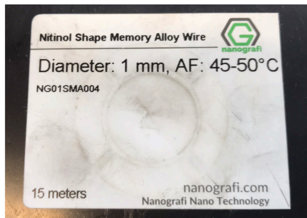
FIGURE 2.30: EXAMPLE PHOTOS OF \pm 5\sim 10^{\circ}\text{C} NITINOL ACTIVATION TEMPERATURE TOLERANCE RANGE FOR TWO DIFFERENT MANUFACTURER/SUPPLIER (NANOGRAFI AND NEXMETAL)
