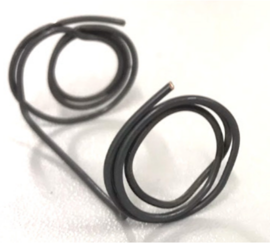
FIGURE 5.29: CURLED U SHAPE TRAINED 1MM DIAMETER SMA WIRE
