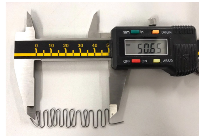
FIGURE E.3: HAND FORMED ZIGZAG SPRING (FIGURE 4.9- B) MADE USING GUIDELINES BEING MEASURED WITH A DIGITAL CALIPER
