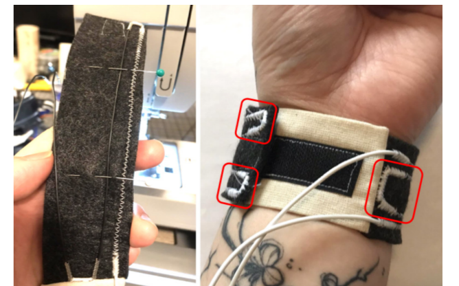
FIGURE 5.40: [LEFT] SEWING PROCESS FOR [RIGHT] THE FINAL WRIST PROTOTYPE. THREE OF THE SOLID CORE ELECTRICAL WIRE CONNECTOR BARS ARE EMPHASIZED.
