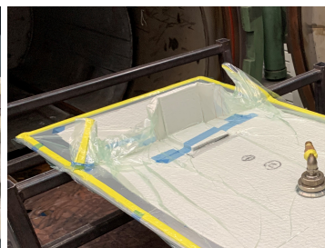
(e) The part was placed inside the autoclave for co-curing
