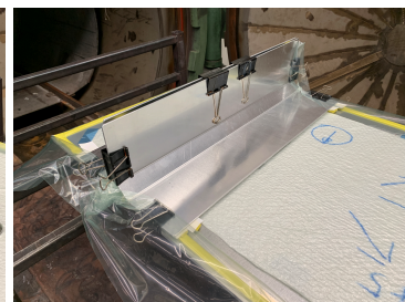
(f) External brackets were used on T-joint 1 (NoInterleaf), but replaced by caul plates in later batches
