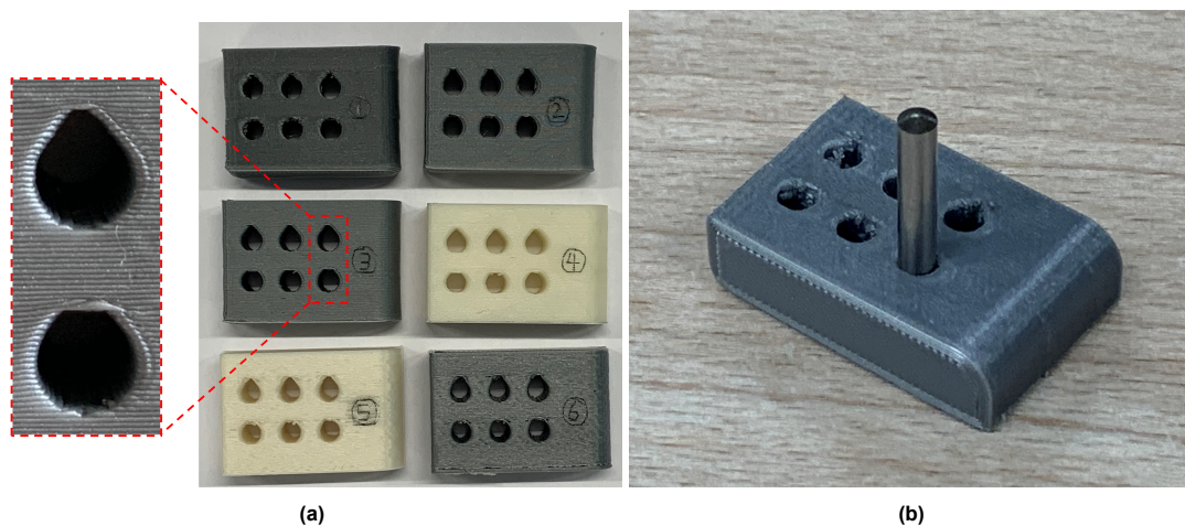
Figure 3.8: 3D printed test pieces for the determination of print parameters
