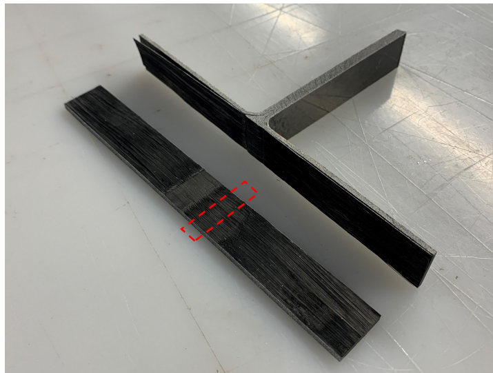
Figure 5.10: T-joint broken for microscopic observation. Box highlights area of observation
