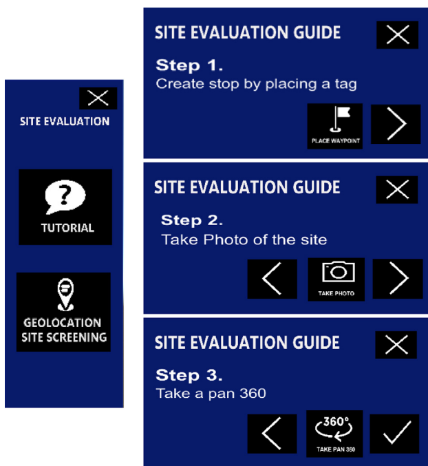
Fig. 5. Site evaluation menu with two options: tutorial and geological site screening (left). The tutorial includes three steps (right): place a waypoint, take a normal photo, and take a panoramic 360° photo.
