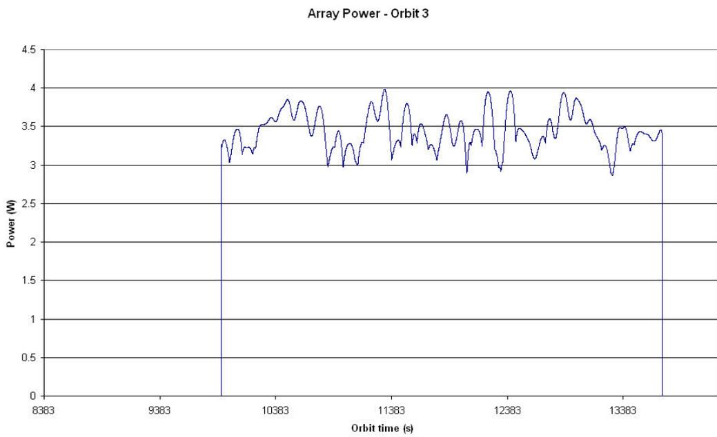
Figure U.3: Scenario 1 - Orbit 3 - Array power
