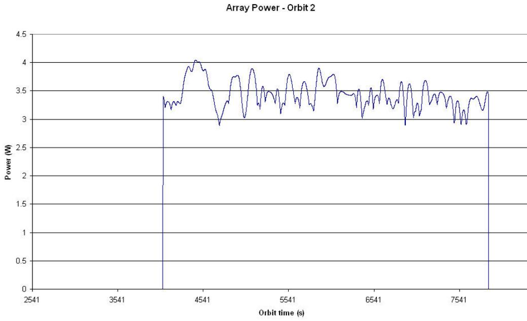
Figure U.2: Scenario 1 - Orbit 2 - Array power
