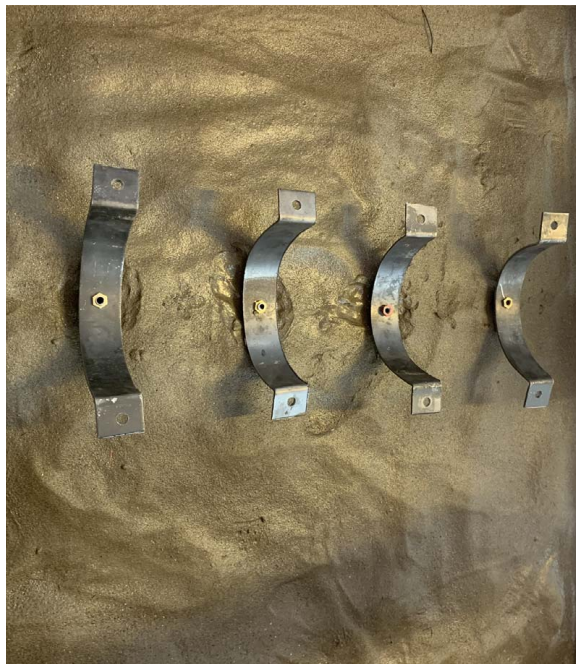
Fig. 5. Lower half of the belts, after screwing to the helical piles to connect to the tunnel.
