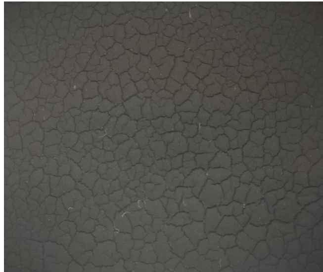
Figure 4.2: Cracked coating film of carbon electrode. Cracks result of residual stress release from colloidal films made by the evaporation of colloidal droplets containing nano particles. Capillary pressures generate tensile stresses normal to the coating film.
