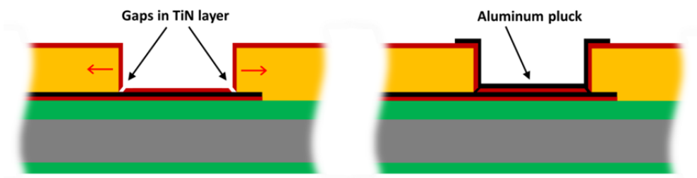
Figure 3.9 (left) Schematic representation of the gaps formed in the TiN layer inside the vias, caused by parylene sidewall retraction as a result of cooling after TiN deposition. (right) Covering the gaps by depositing and patterning a layer of aluminum to form an “Al plug” inside the vias.
