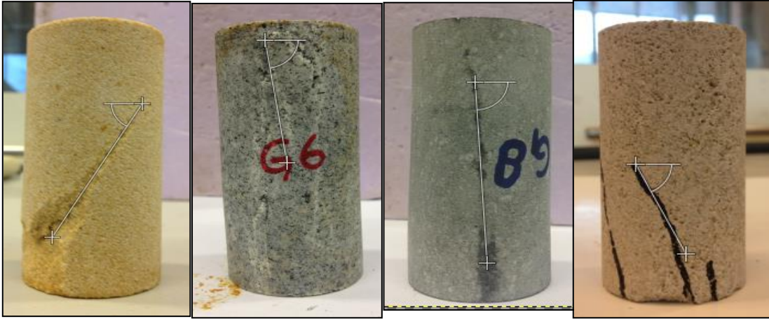
Figure 28. Fracture angle at zero confining pressure. From left to right: BB Sandstone, Granite, Belgium LS, Indiana LS
