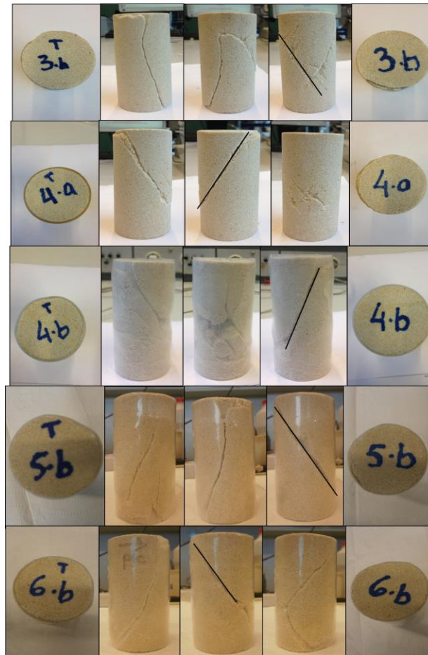
Figure 81. Example of BB Sandstone after the Confined pressure test (different number corresponds to different confining pressure)
