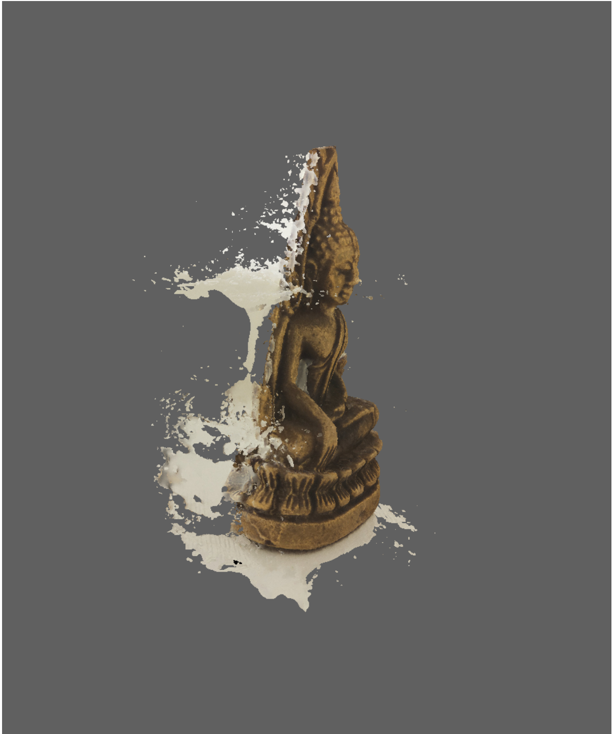
Figure 7.10: 3D-image created with the "minimal" settings. 10 Minutes were needed to acquire the photographs, and 20 minutes were needed to post-process the photographs to create the 3D-image. Click the figure to be able to move the 3D-image.
