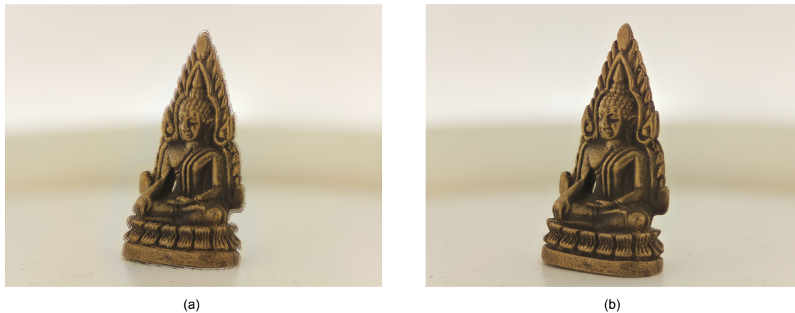
Figure 7.8: The result of focus stacking the photographs of the object with two different methods. (a) The weighted-average method. (b) The Laplacian pyramid method.
