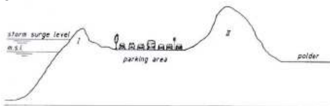
Figure 5: Situation in which erosion will not be controlled
