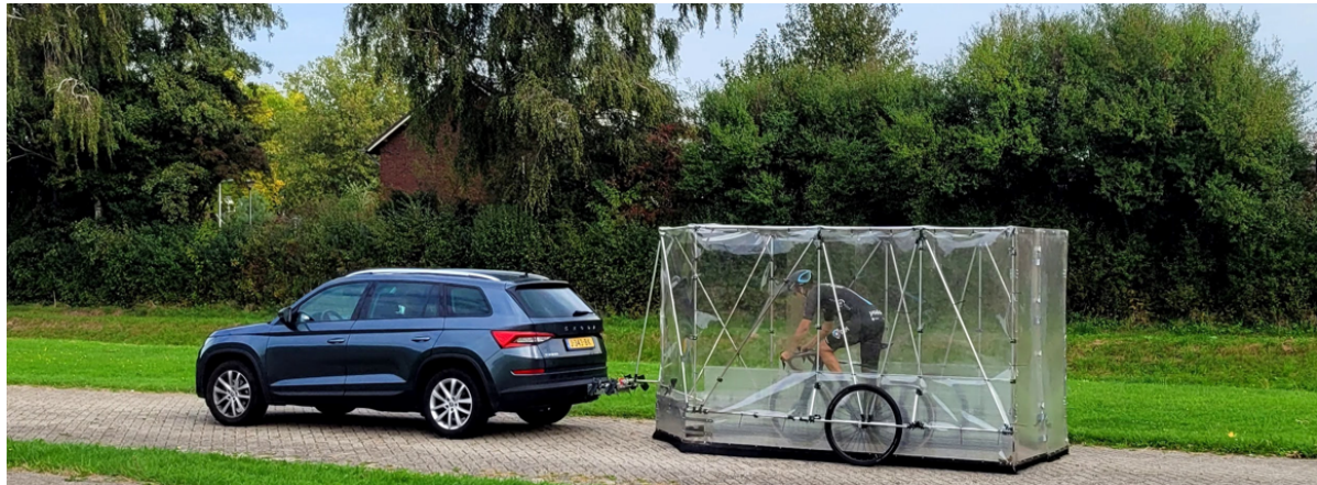
Figure 4.6: Test setup for the bike trailer measurement
