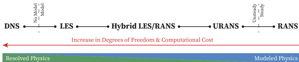
Figure 1.2: Turbulence modeling approaches spectrum
