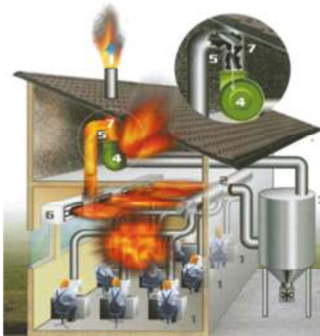
Figure 3: Aluminum dust explosion in a grinding room (ISSA, 2005)
