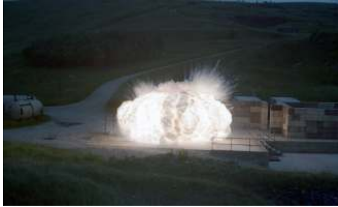
Figure 10. Vented aluminum dust explosion test illustrating the very high emissivity of aluminum flames (Holbrow et al., 2000) ©Crown Copyright, Contains public sector information published by the Health and Safety Executive and licensed under the Open Government Licence Courtesy of Paul Holbrow, Health and Safety Laboratory, UK
