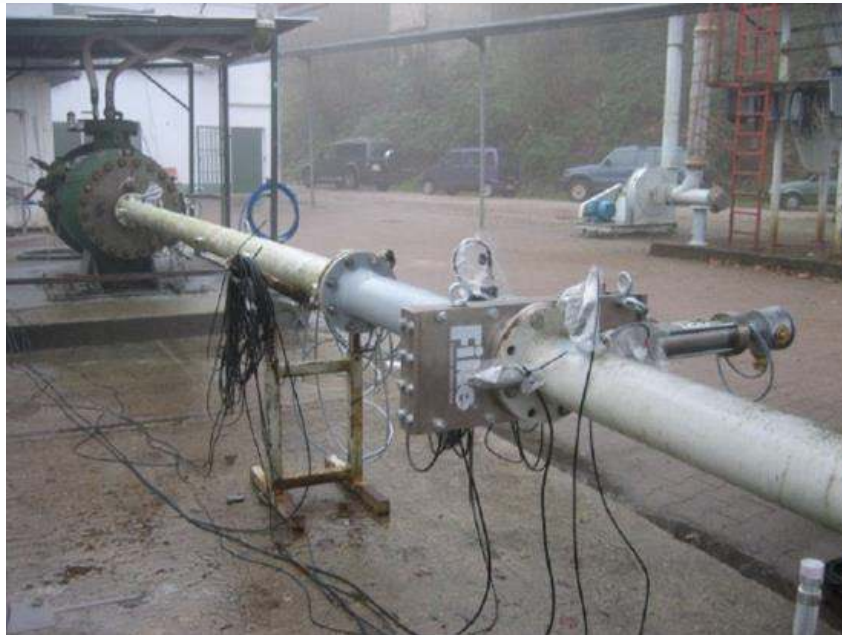
Figure 13: Mechanical explosion isolation of an aluminum dust ( K_{St} = 680 \text{ bar.m/s} ) deflagration initiated in a 1-m 3 contained vessel (Taveau et al., 2013)
