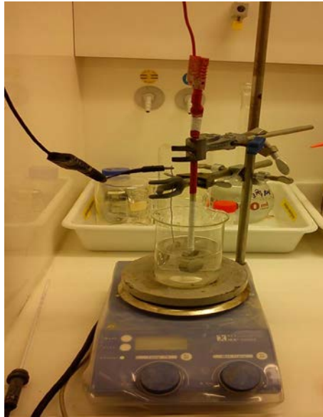
Figure 16 PEO set up used for preparing PEO-Ca surface
